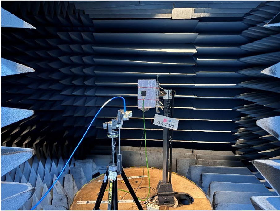
Photograph 5: EUT test setup in the fully anechoic chamber
