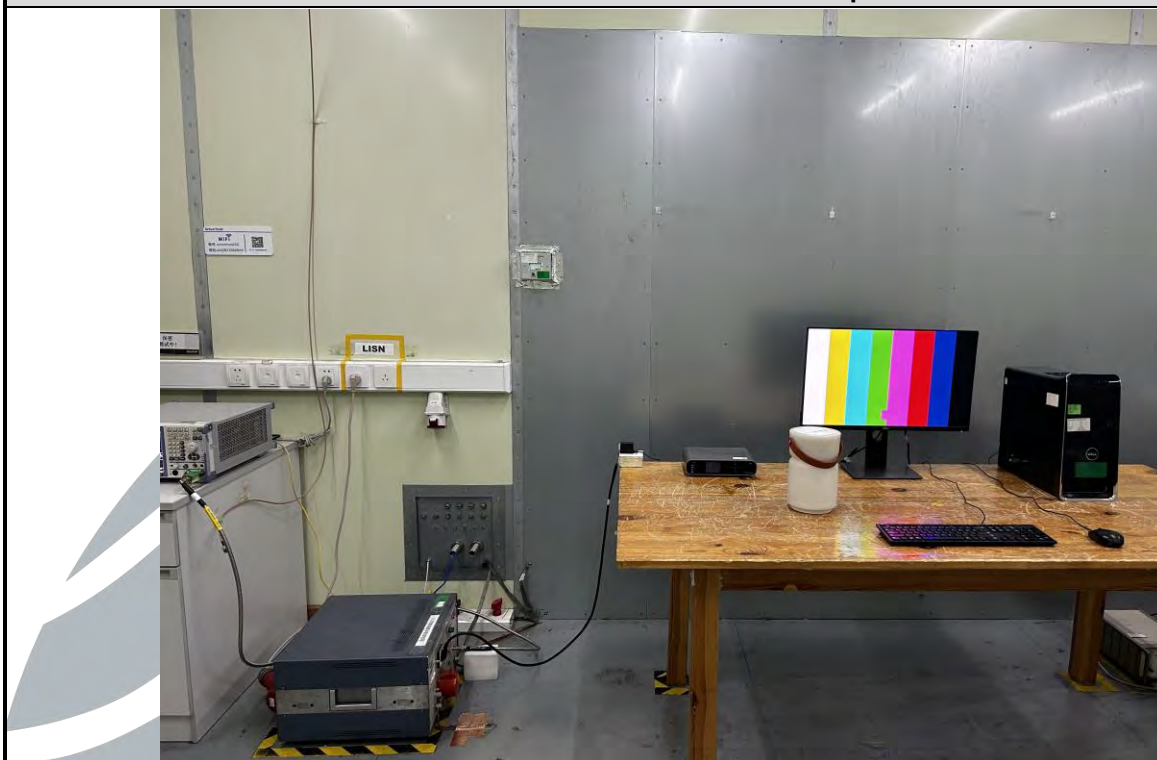
Conducted Emission Test Setup
