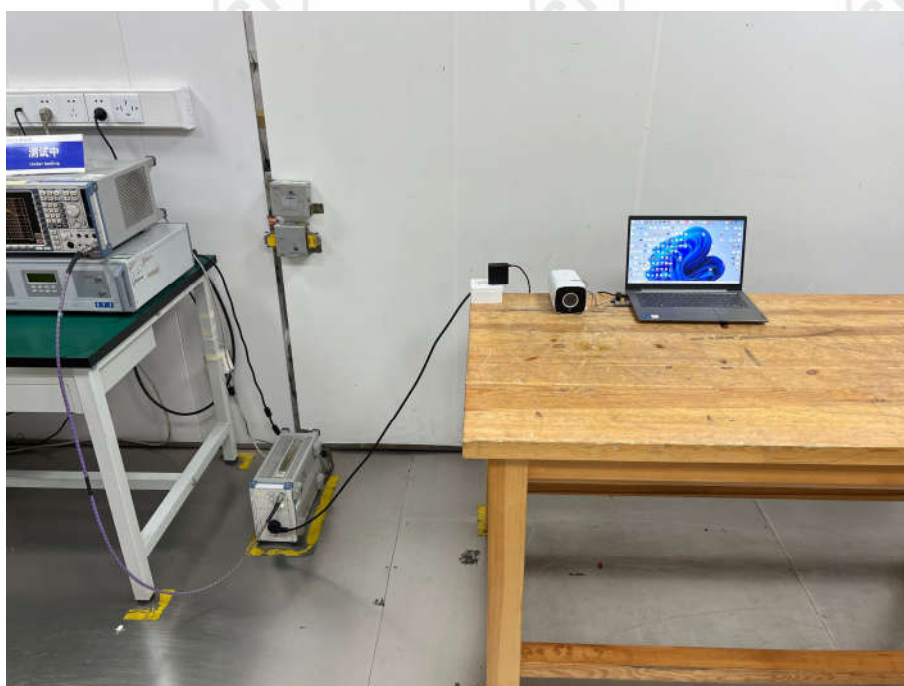
Conducted Emissions Test Setup
