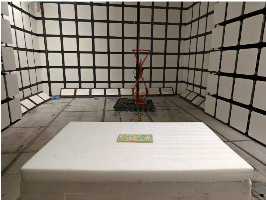
Radiated Emissions View (30 MHz- 1 GHz)
