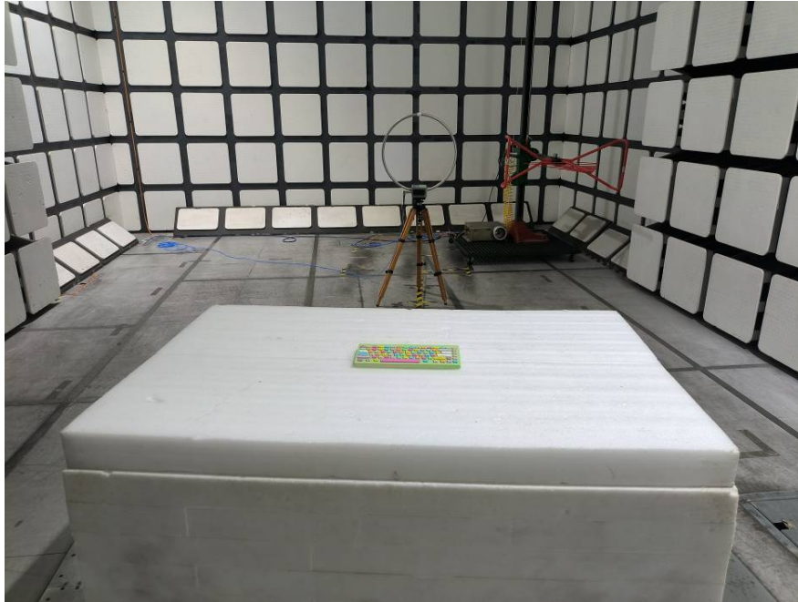
Radiated Emissions View (9 kHz- 30 MHz)
