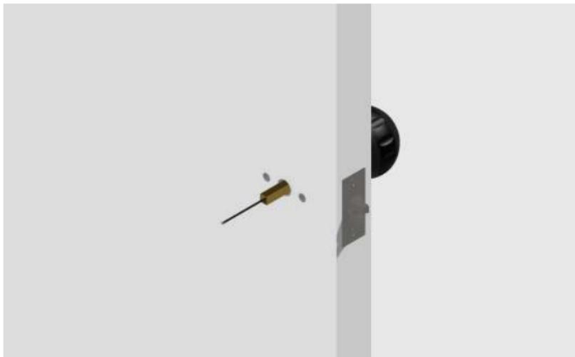
03. Insert the exterior assembly into the door hole.
