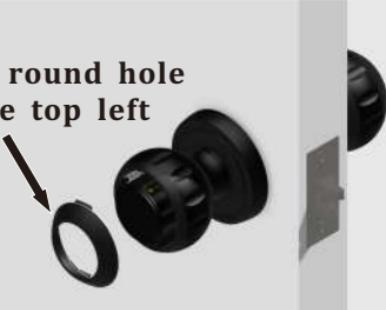
07. To install the battery cover retaining ring, make sure that the small round hole is in the upper left corner, and note that the small round hole must be in the same direction as the rear circuit board. If it is in the wrong position, the clip will not be secured. The structure of the two buckles is different, and it cannot be fixed at any position.
