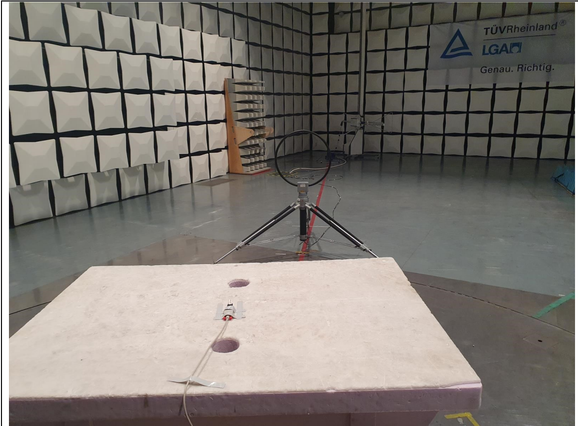
Test Setup: Radiated Measurements (9 kHz - 30 MHz) Parallel polarization EUT Side
