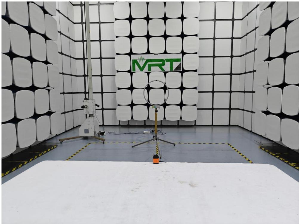
Description: Radiated Spurious Emissions Test Setup for 30MHz ~ 1000MHz
