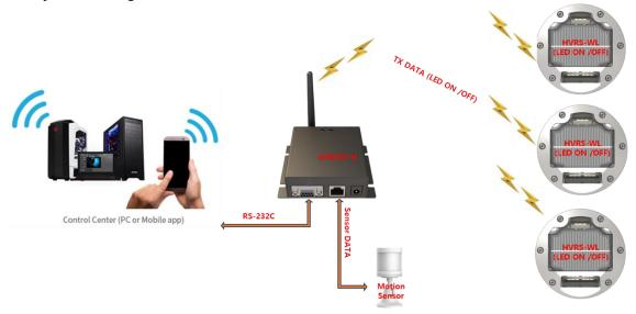
The GIWICS system turns on the LED when the signal unit (HVRS-WL) receives the data transmitted through the RF modem (GIWICS-H). The purpose is to operate the HVRS-WL by receiving sensor data through the external input/output of the RF modem (GIWICS-H).
