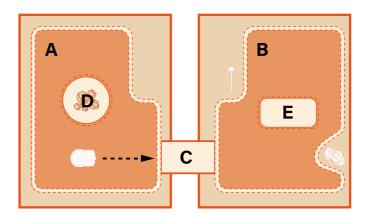
The machine will plan the cutting paths automatically The charging station and RTK base station are located outside the boundary wire, and the charging station is next to the border.
