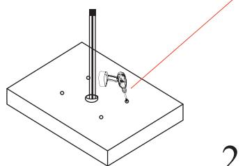
Drive the expansion screw into the cement pier.
