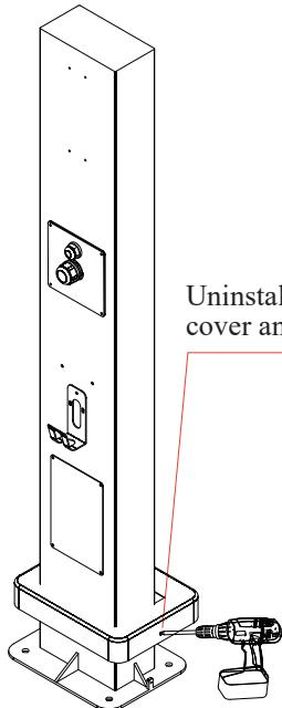
Aligned the screws of pedestal with the ones in cement pier and tight them.
