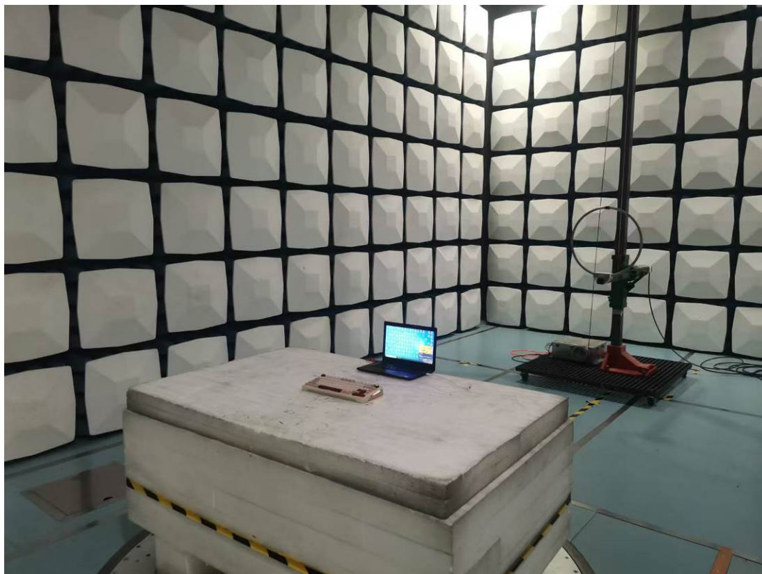
Radiated Emission 9k-30MHz Perpendicular View
