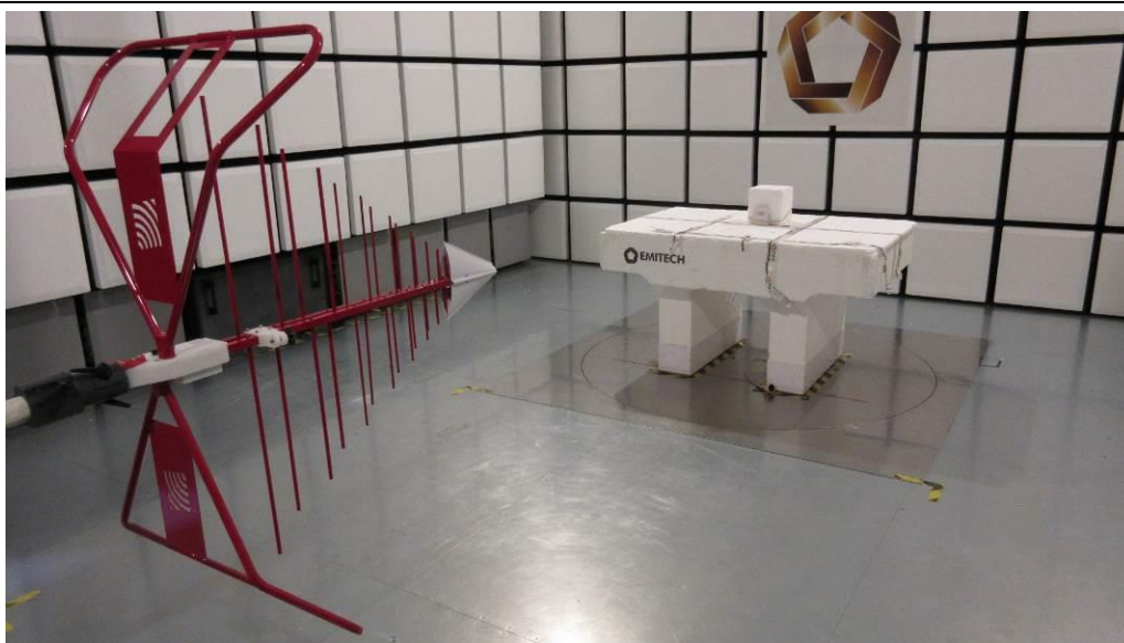
TEST SETUP PHOTO(S) - 30 MHz TO 1 GHz
