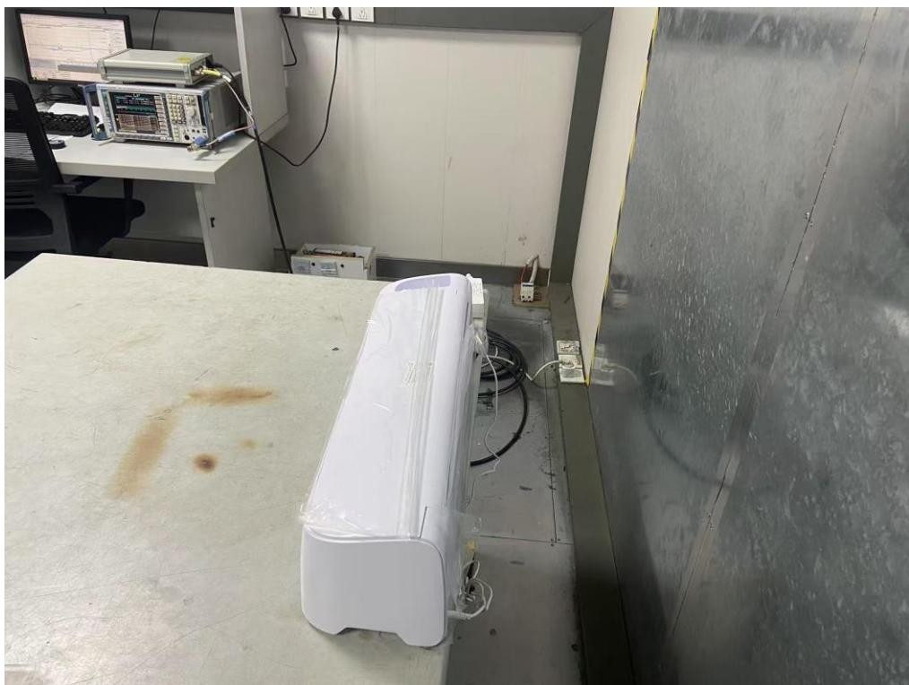
**Radiated Test (Below 1GHz)**
