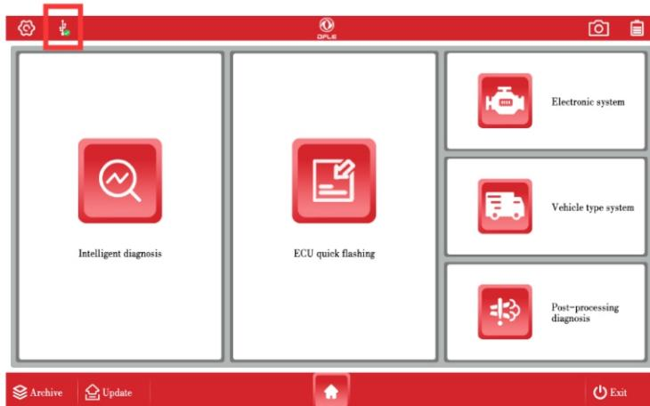
**Bluetooth connection:** Insert the diagnostic apparatus into the OBD plug of the vehicle, turn on the vehicle key, turn on the bluetooth, search for the bluetooth, make sure bluetooth name and device serial number are consistent then click pairing. As shown in the figure below:
