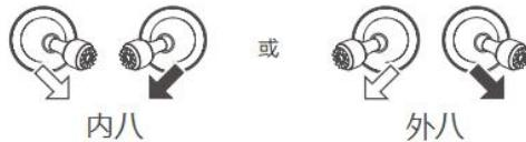
Both the inner eight and outer eight can be unlocked and locked. It is recommended to unlock the inner eight and lock the outer eight.
