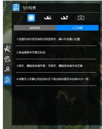
Manual inspection of structural connections and the current and actual orientation of the magnetic compass, with a deviation of generally within 5 degrees, is normal.
