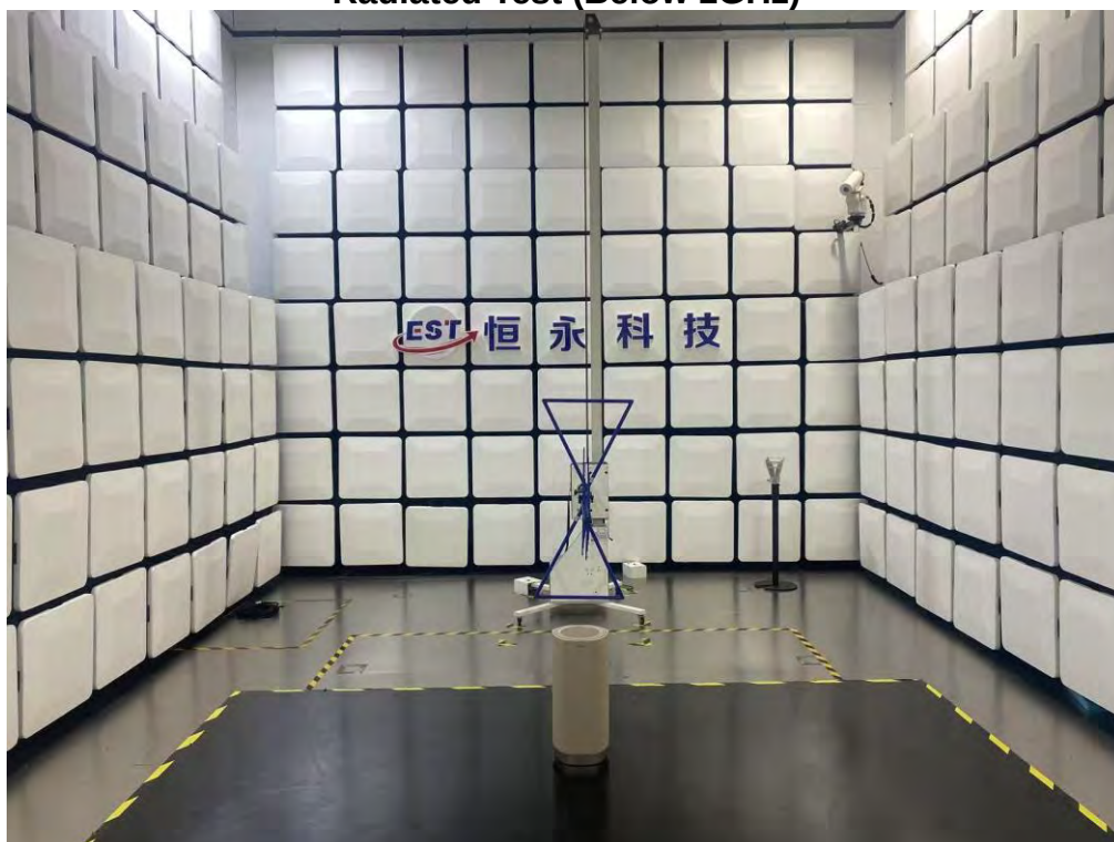
Radiated Test (Below 1GHz)
