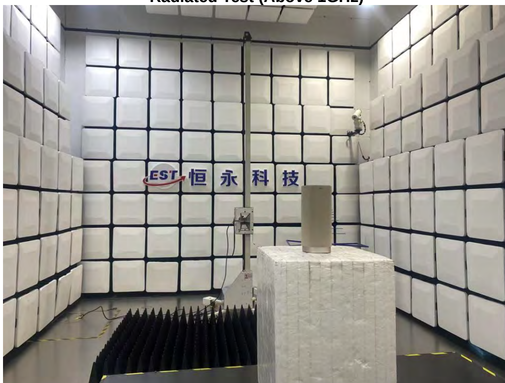
Radiated Test (Above 1GHz)
