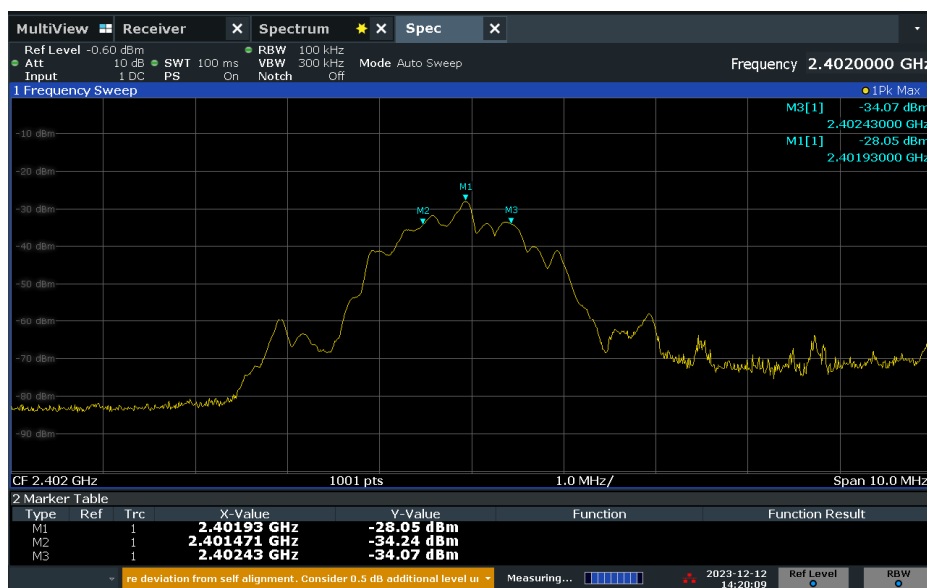
Figure 2-3 – 6dB Bandwidth – High Channel – 1Mps
