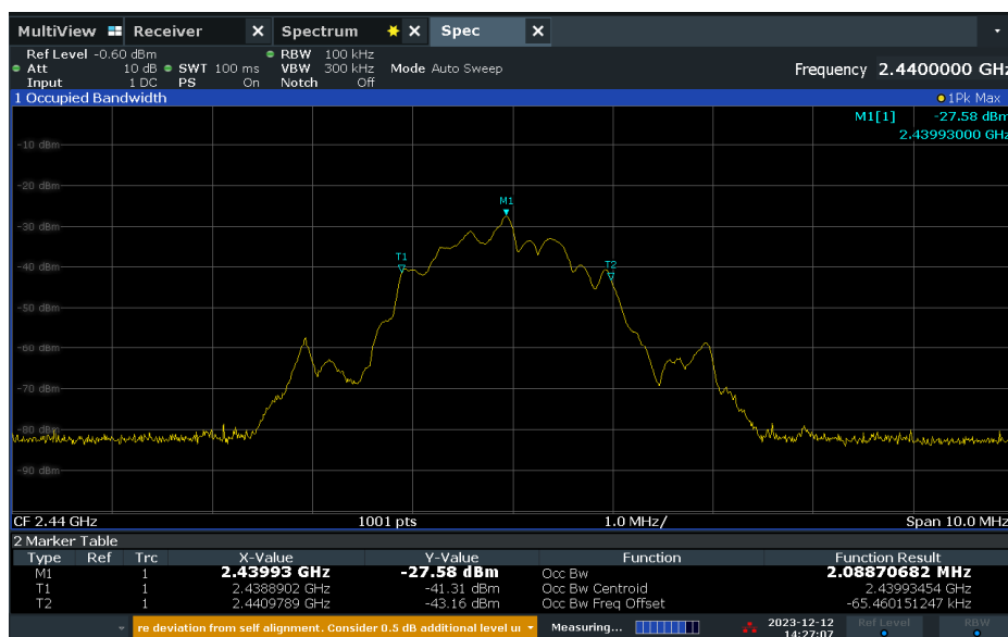
Figure 2-11 – 99% Bandwidth – Middle Channel – 2Mps
