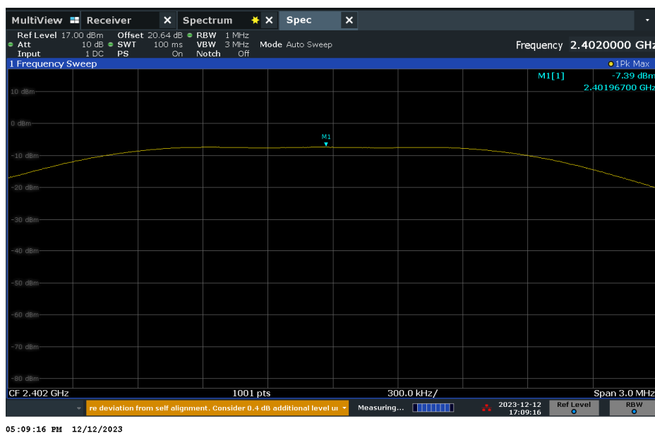
Figure 2-16 – Peak Conducted Output Power – Low Channel – 2Mbps
