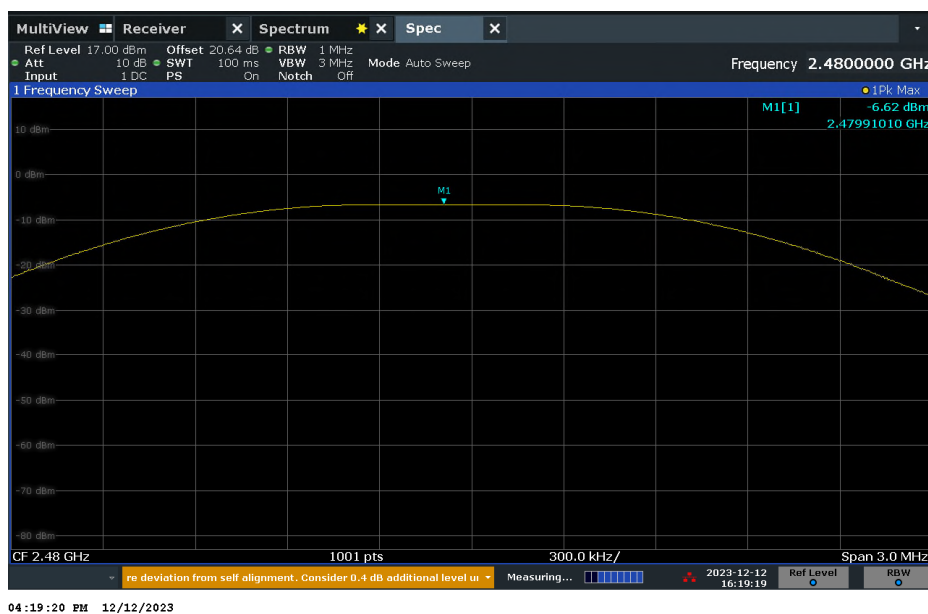
Figure 2-15 – Peak Conducted Output Power – High Channel – 1Mbps
