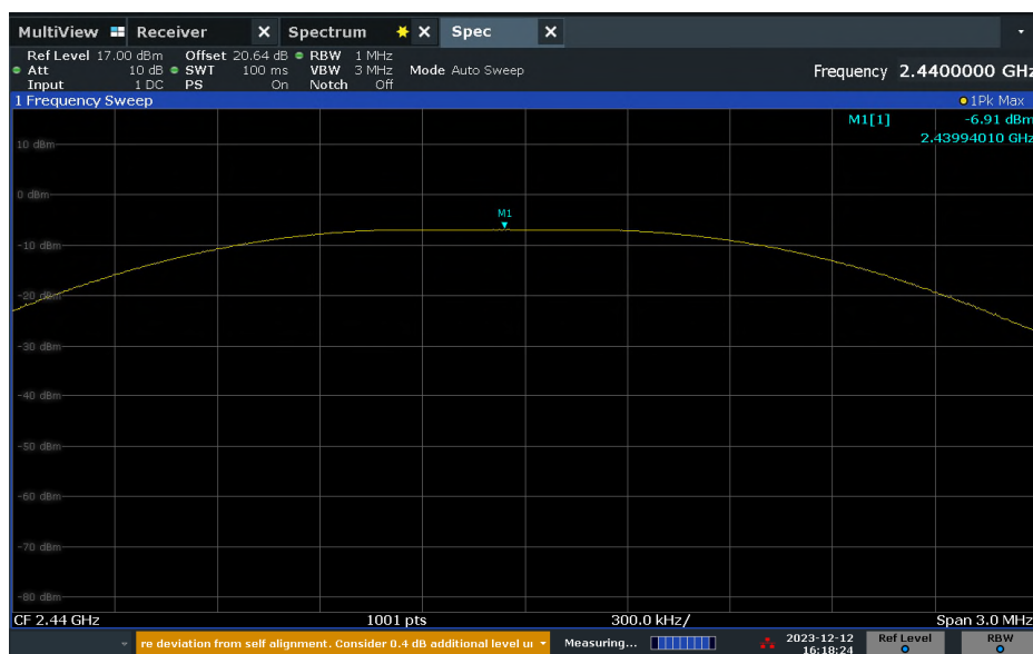
Figure 2-13 – Peak Conducted Output Power – Low Channel – 1Mps
