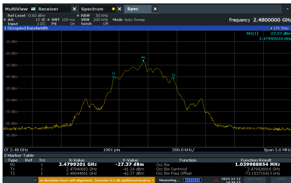
Figure 2-9 – 99% Bandwidth – High Channel – 1Mps
