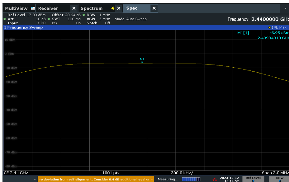
Figure 2-17 – Peak Conducted Output Power – Middle Channel – 2Mps
