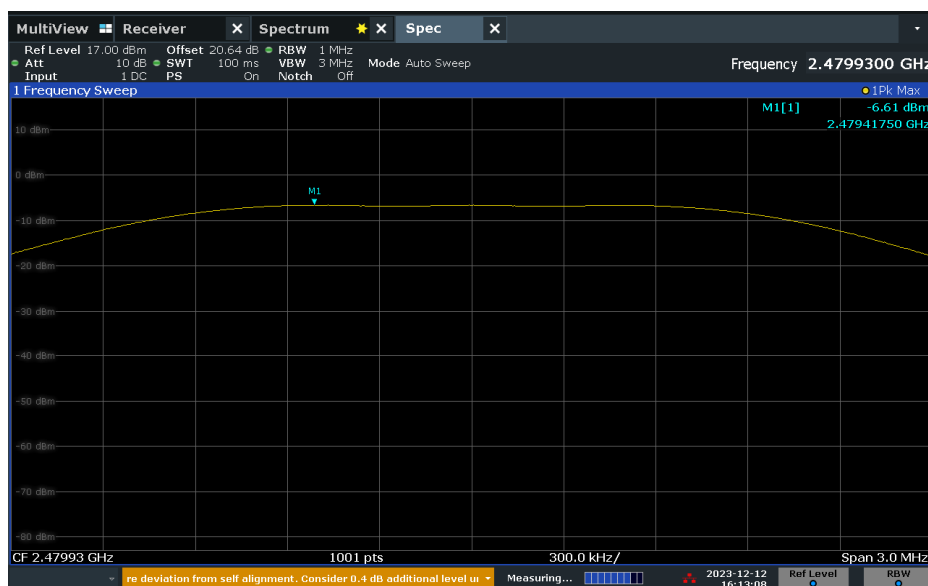
Figure 2-17 – Peak Conducted Output Power – Middle Channel – 2Mps
