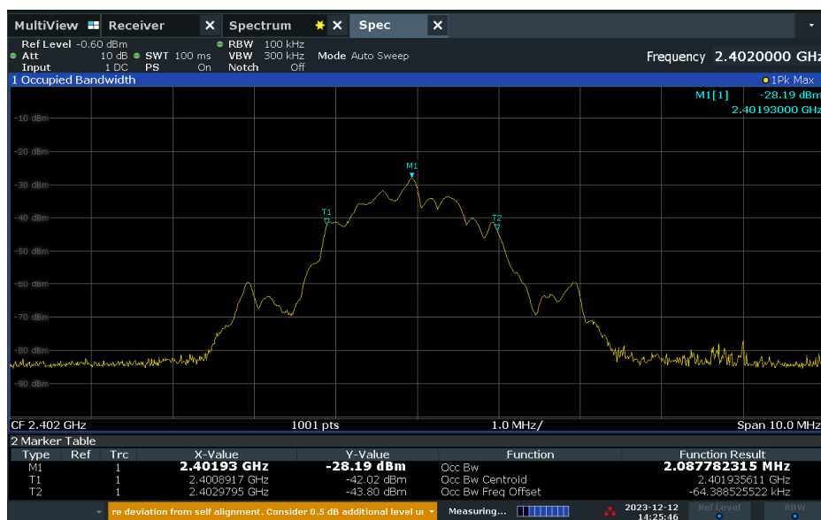
Figure 2-9 – 99% Bandwidth – High Channel – 1Mps
