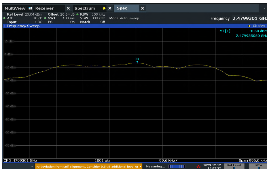
Figure 2-21 – Peak Conducted Output Power – High Channel – 1Mbps
