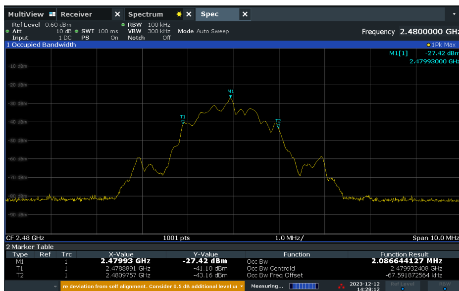
Figure 2-11 – 99% Bandwidth – Middle Channel – 2Mps
