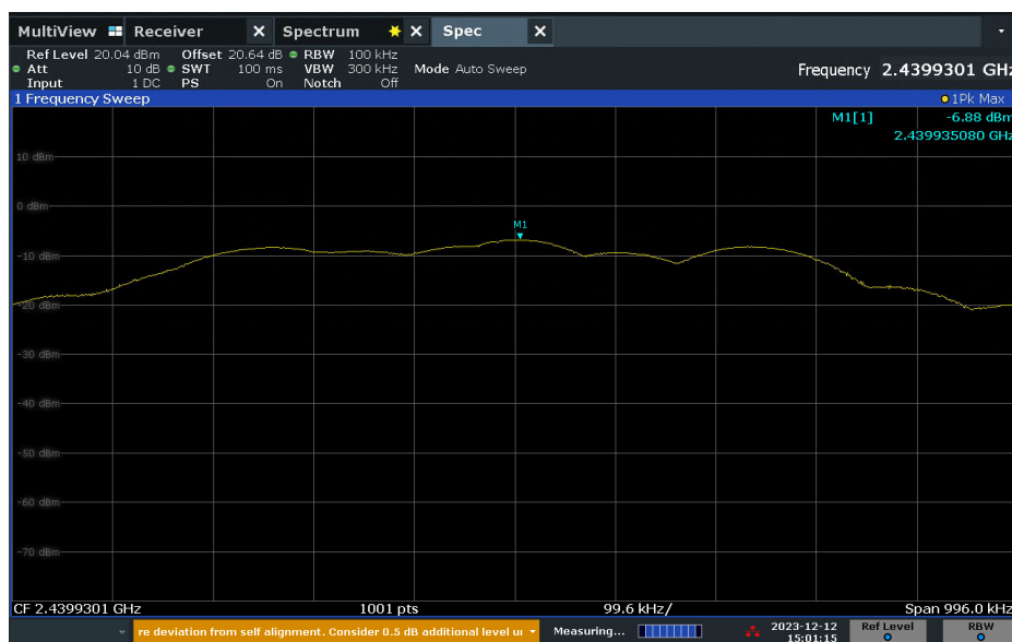
Figure 2-19 – Peak Conducted Output Power – Low Channel – 1Mps
