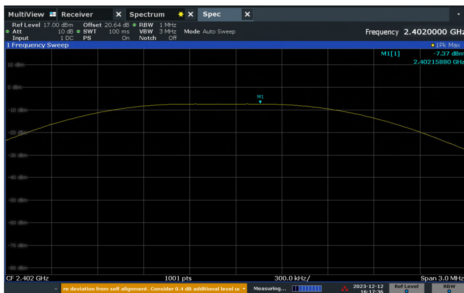
Figure 2-13 – Peak Conducted Output Power – Low Channel – 1Mps
