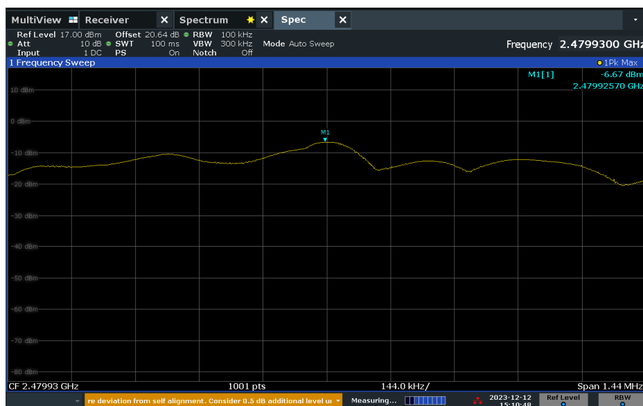
Figure 2-23 – Peak Conducted Output Power – Middle Channel – 2Mps
