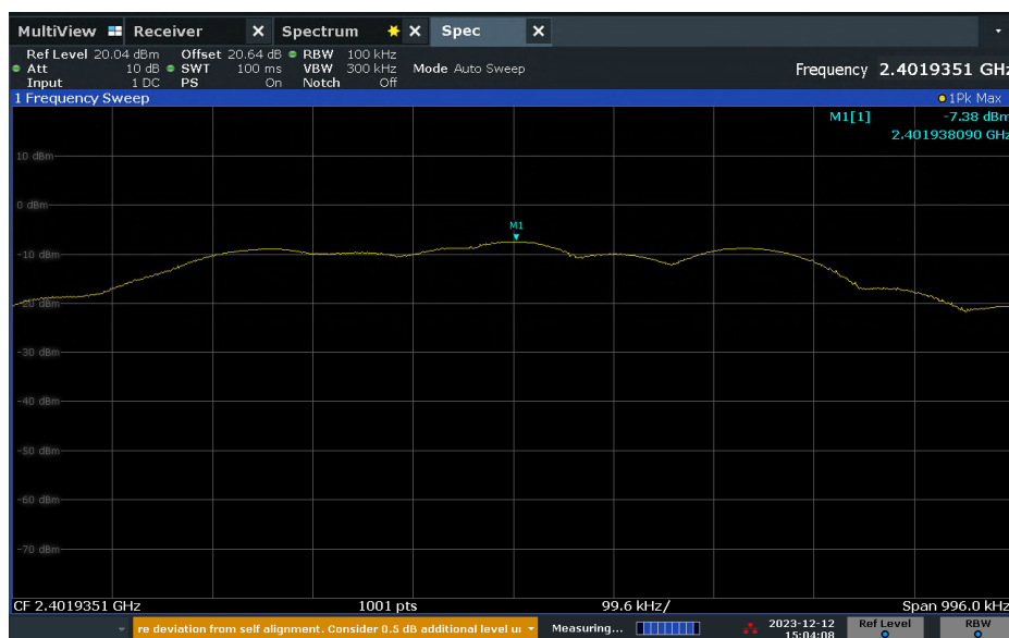
Figure 2-19 – Peak Conducted Output Power – Low Channel – 1Mps
