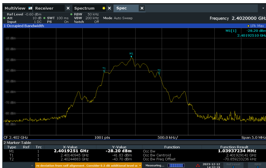
Figure 2-7 – 99% Bandwidth – Low Channel – 1Mps
