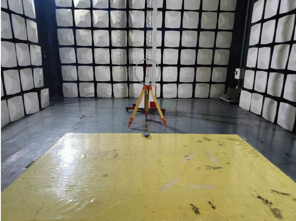
Test Photo Radiated emission (Below 30MHz)
