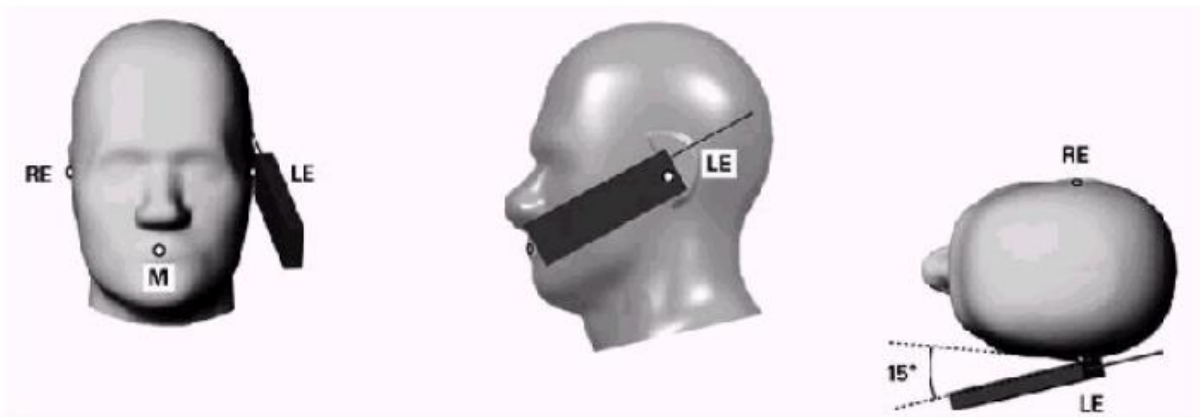
Figure 7.3.1 – Tilt position of the wireless device on the left side of SAM
