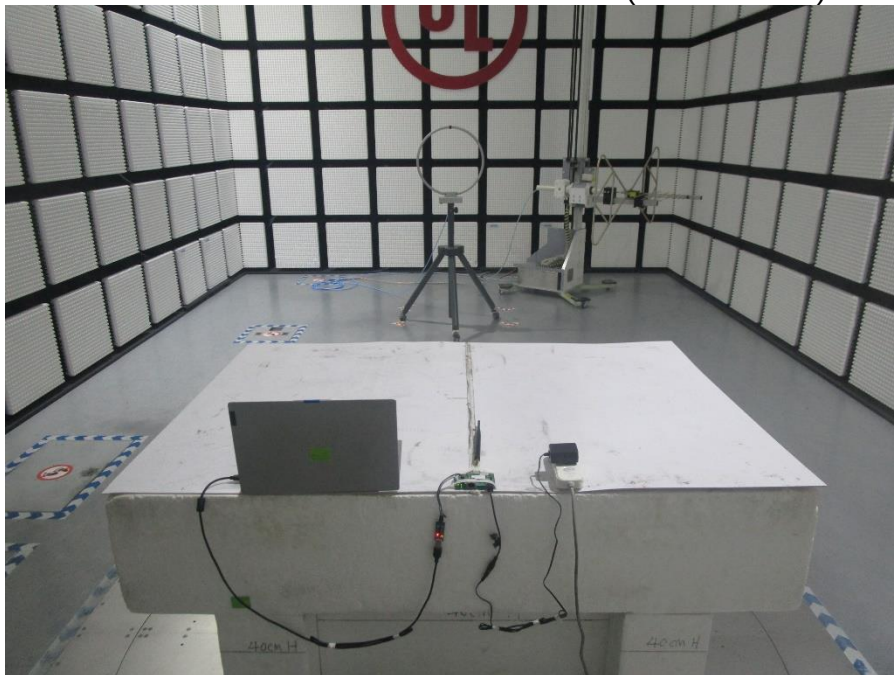
RADIATED RF MEASUREMENT SETUP (Below 30MHz)
