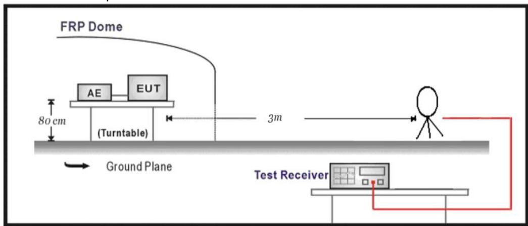
Below 1GHz Test Setup:
