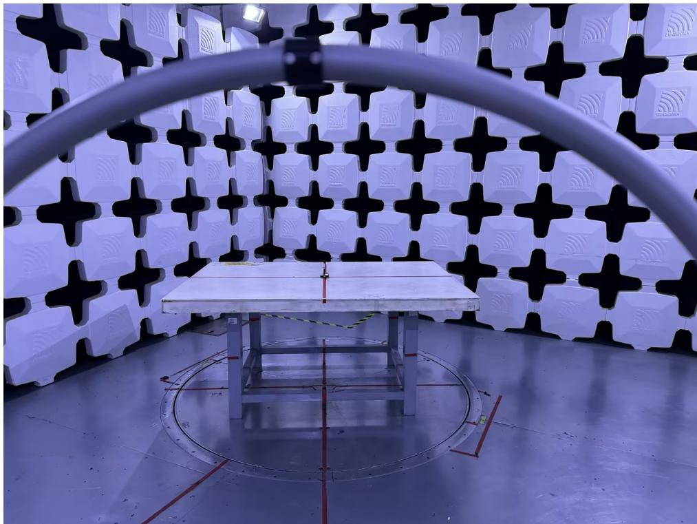
**Radiated Emissions Test Photos****30 MHz to 1 GHz**
