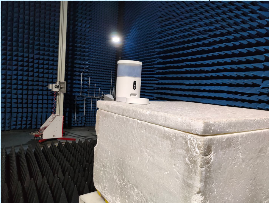
Radiated Emission Above 1GHz Test Setup
