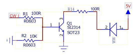
CW\_I is the PWM output pin of the module pure white light, Q1 is the MOS tube, WW is the LED lamp bead, and the other 4-way lamp drive circuit is the same as the design method of this way, please see more detailed design original document on web disk data:
