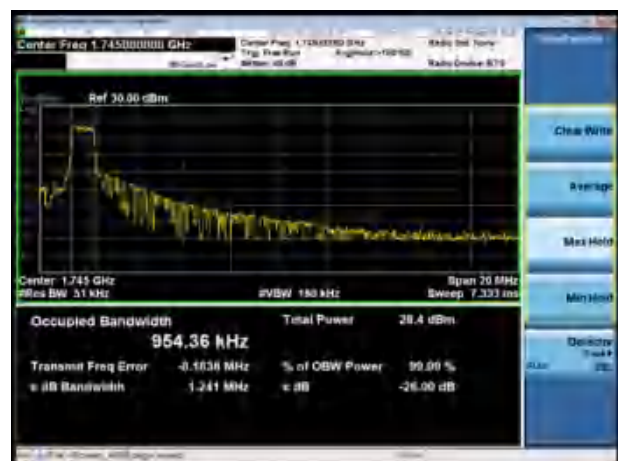
LTE Band 66 16QAM 20MHz CH-Middle
