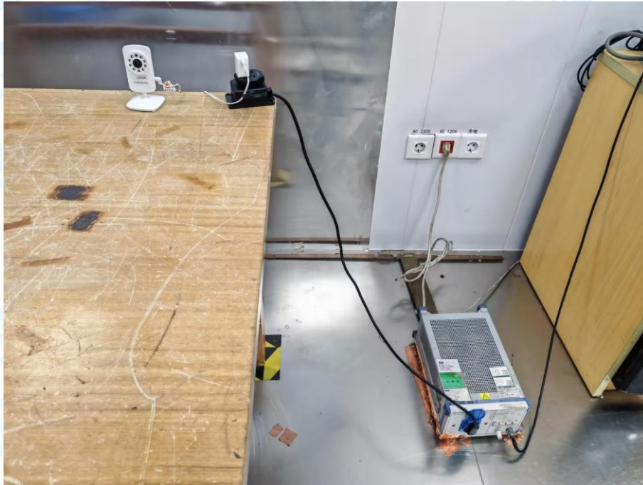
Photo of Setup for Radiated Emission (30MHz~1GHz)
