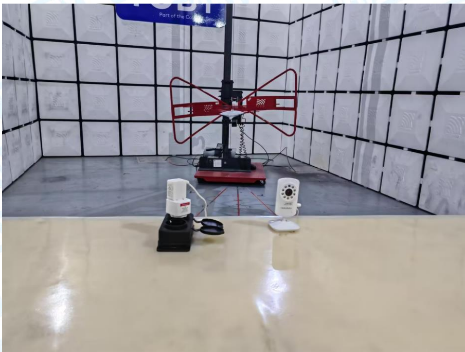
Photo of Setup for Radiated Emission (30MHz~1GHz)
