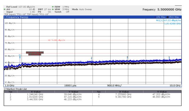
Limit according to FCC Part 15C, Section 15.209:
