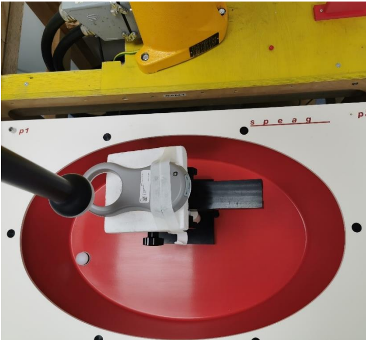
Figure 18. Test position 3, separation distance 100mm
