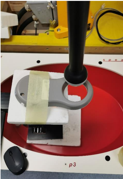
Figure 8. Test position 3, separation distance 0mm
