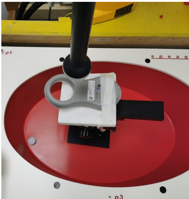
Figure 19. Test position 4, separation distance 100mm
