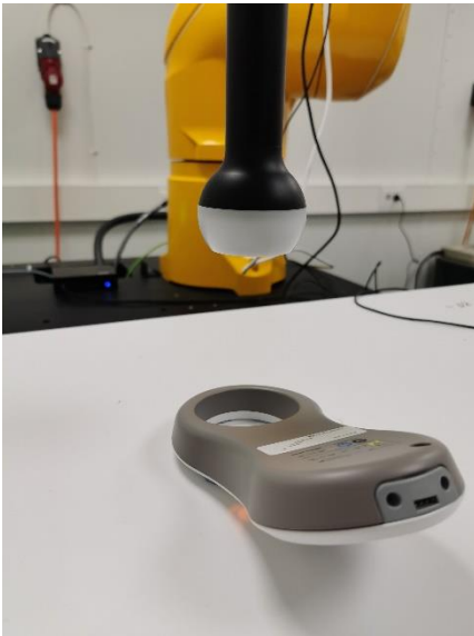
Figure 20. Test position 5, separation distance 100mm
