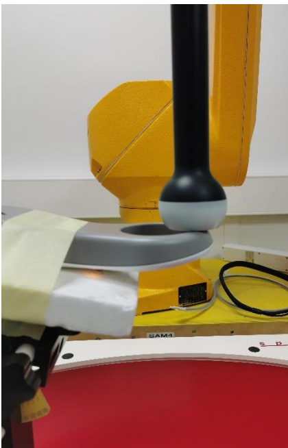
Figure 7. Test position 2, separation distance 0mm
