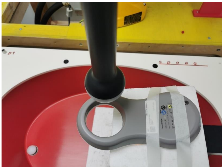
Figure 11. Test position 1, separation distance 30mm
