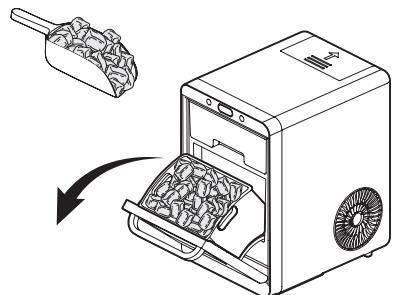
Place the ice basket in the limit slot, or it will fall into the inside of the ice maker.
