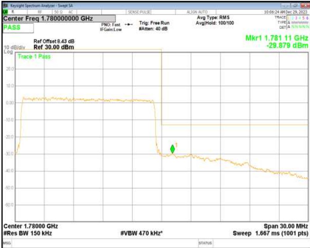
Band66 QPSK BW=20MHz Channel=132072 RB Size=100 Position=#0
