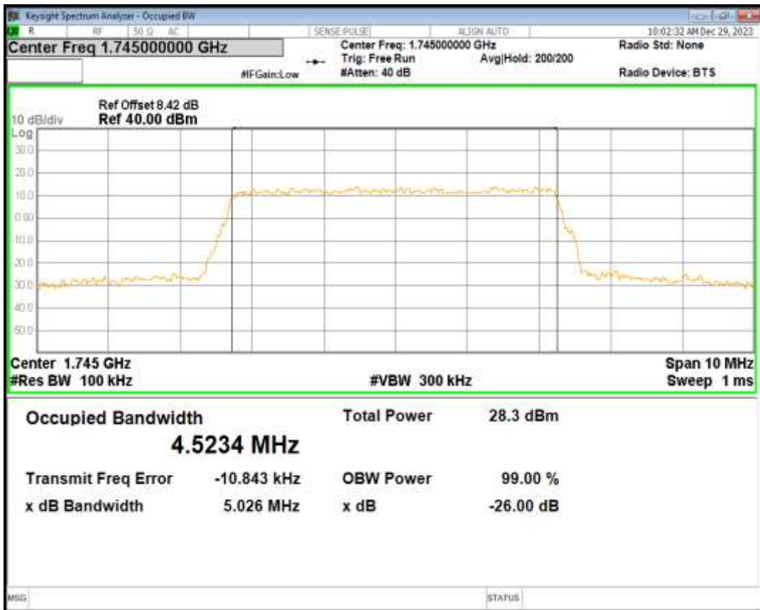
Band66 16QAM BW=5MHz Channel=132647 RB Size=25 Position=#0
