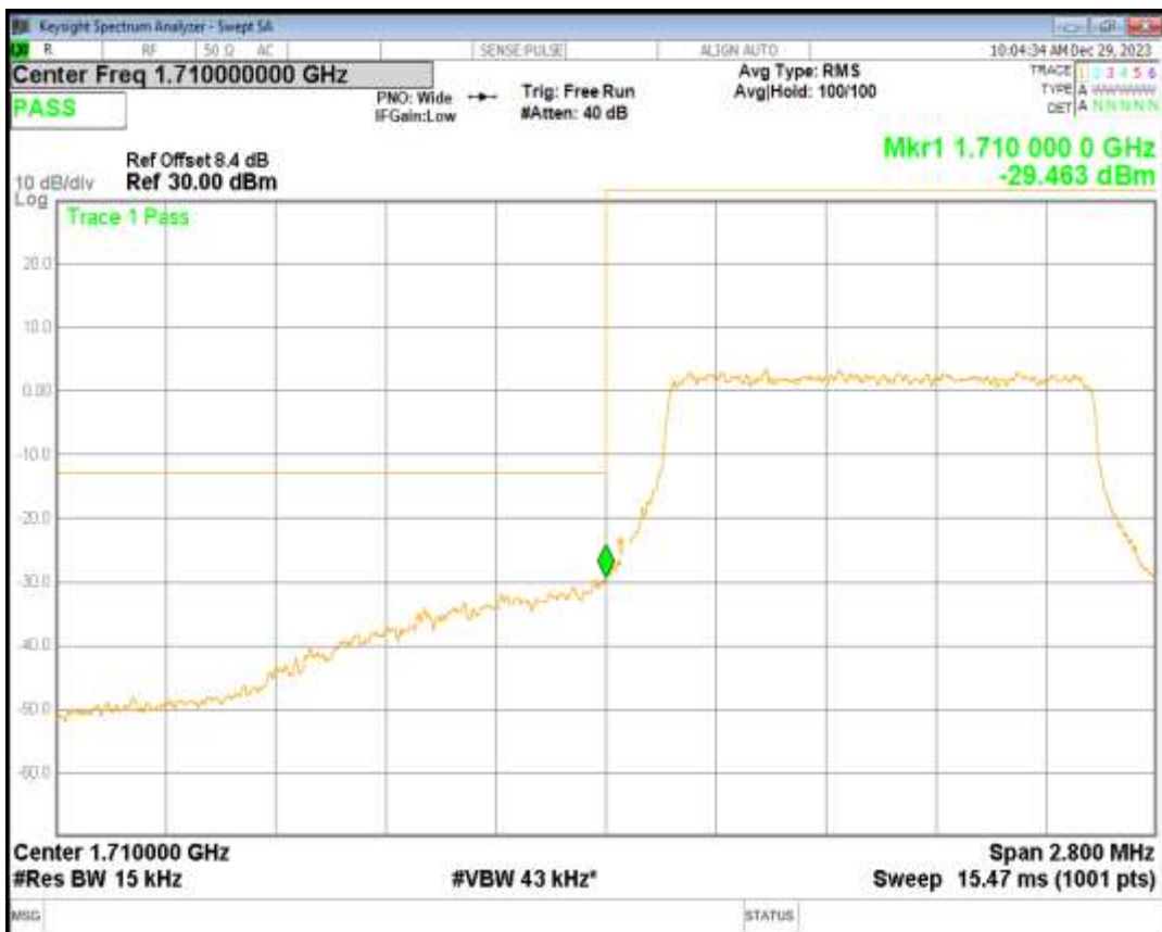
Band66 16QAM BW=1.4MHz Channel=132665 RB Size=6 Position=#0
