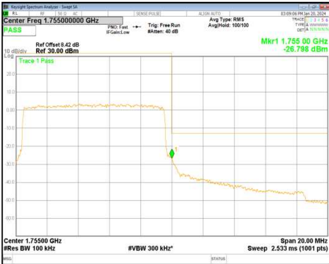
Band4 QPSK BW=15MHz Channel=20025 RB Size=75 Position=#0
