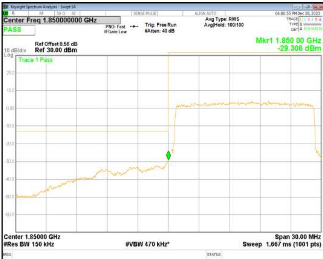
Band2 QPSK BW=15MHz Channel=19125 RB Size=75 Position=#0
