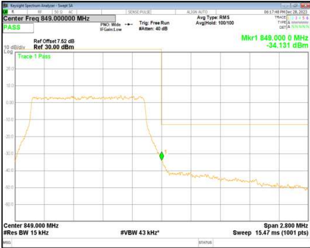
Band5 16QAM BW=10MHz Channel=20450 RB Size=50 Position=#0
