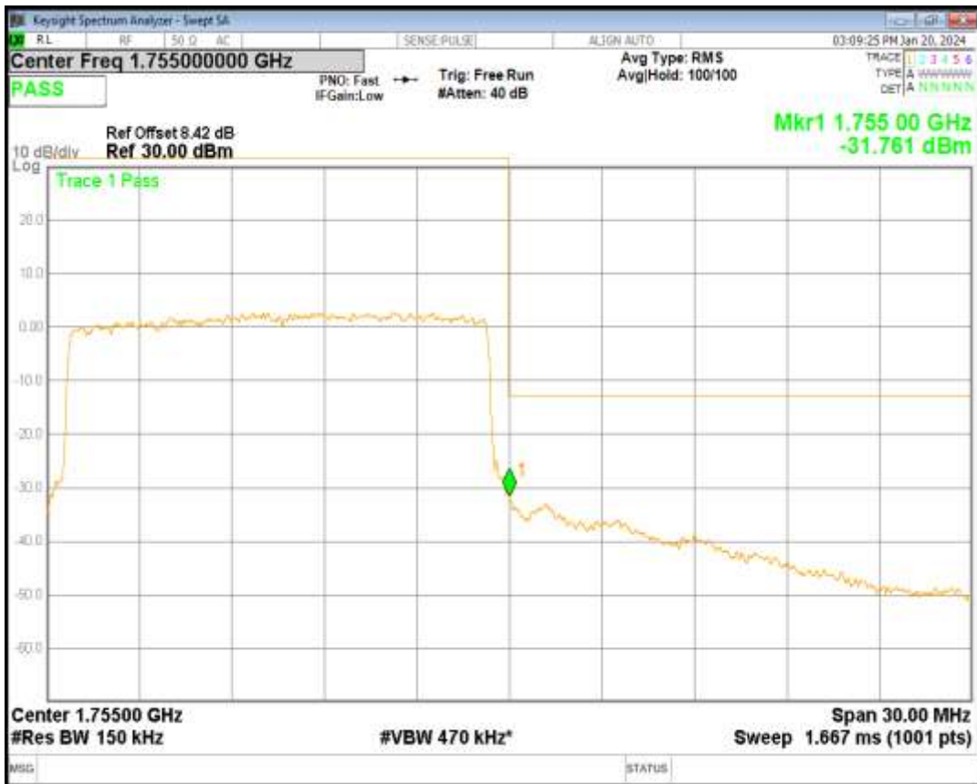
Band4 16QAM BW=20MHz Channel=20050 RB Size=100 Position=#0
