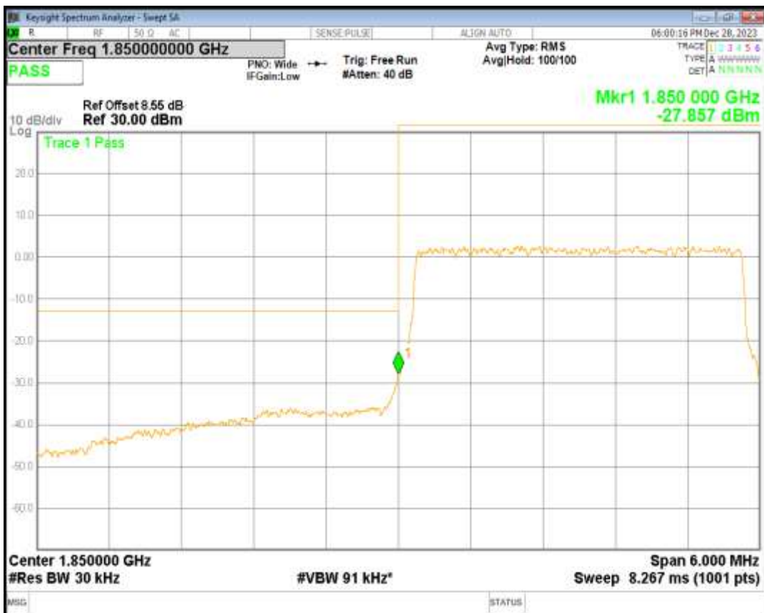
Band2 16QAM BW=3MHz Channel=19185 RB Size=15 Position=#0
