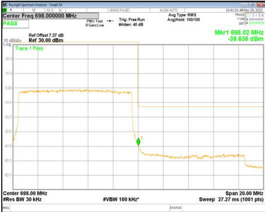
Band71 QPSK BW=15MHz Channel=133197 RB Size=75 Position=#0
