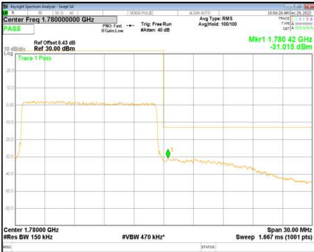
Band66 16QAM BW=20MHz Channel=132072 RB Size=100 Position=#0
