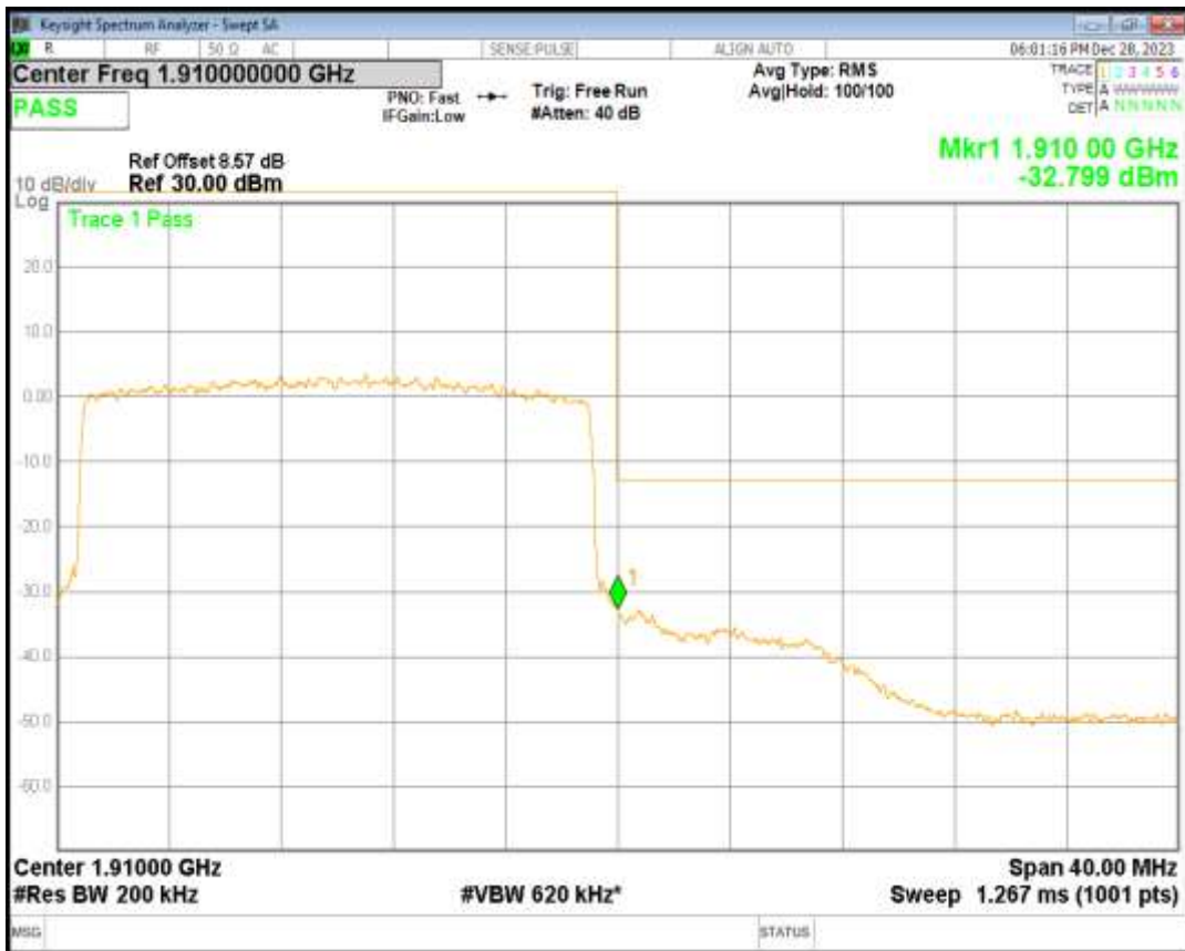
Band2 16QAM BW=3MHz Channel=18615 RB Size=15 Position=#0
