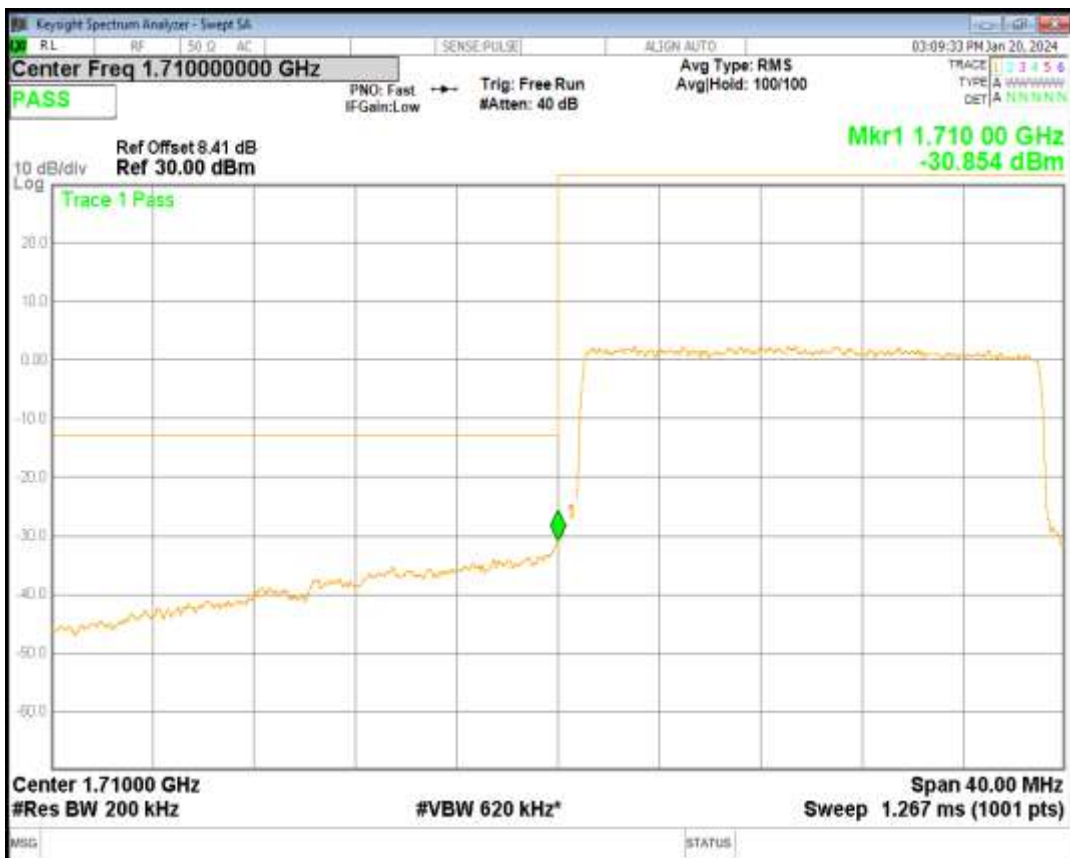
Band4 16QAM BW=20MHz Channel=20300 RB Size=100 Position=#0
