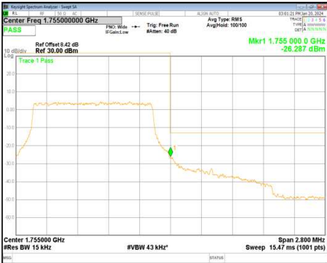
Band4 16QAM BW=5MHz Channel=20375 RB Size=25 Position=#0
