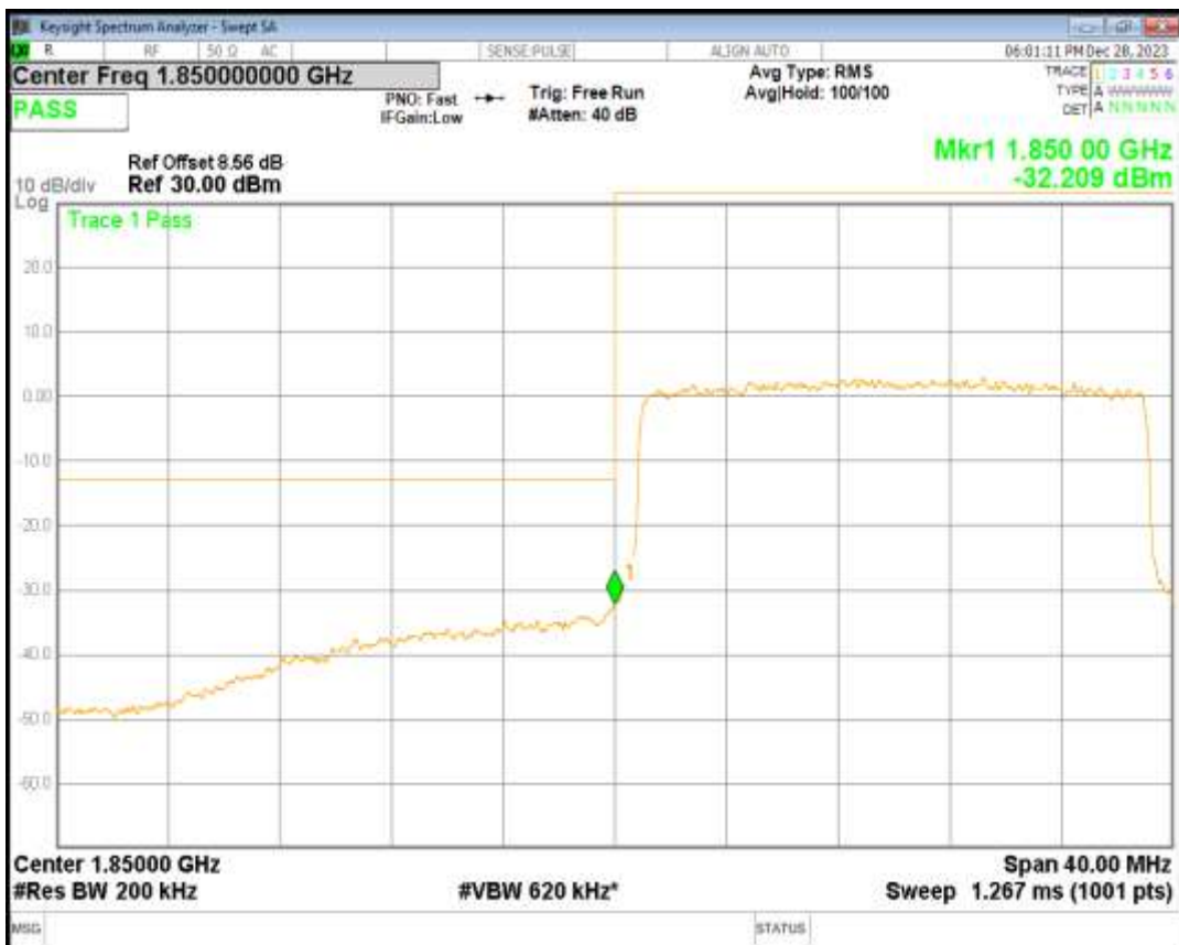
Band2 16QAM BW=20MHz Channel=19100 RB Size=100 Position=#0
