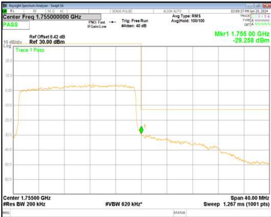
Band4 QPSK BW=5MHz Channel=19975 RB Size=25 Position=#0
