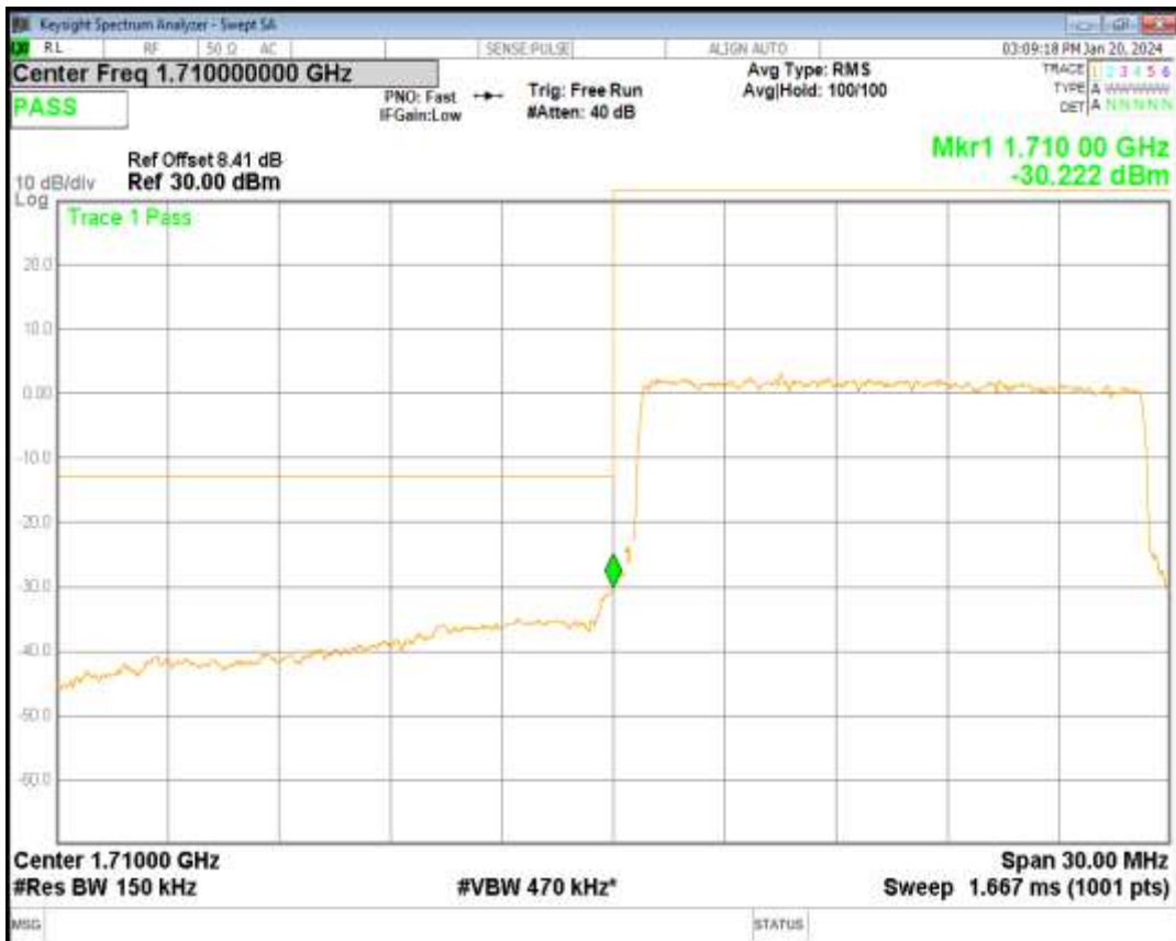
Band4 16QAM BW=15MHz Channel=20325 RB Size=75 Position=#0
