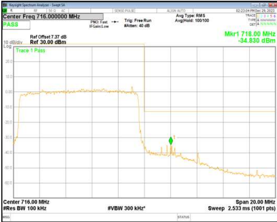
Band17 16QAM BW=5MHz Channel=23755 RB Size=25 Position=#0
