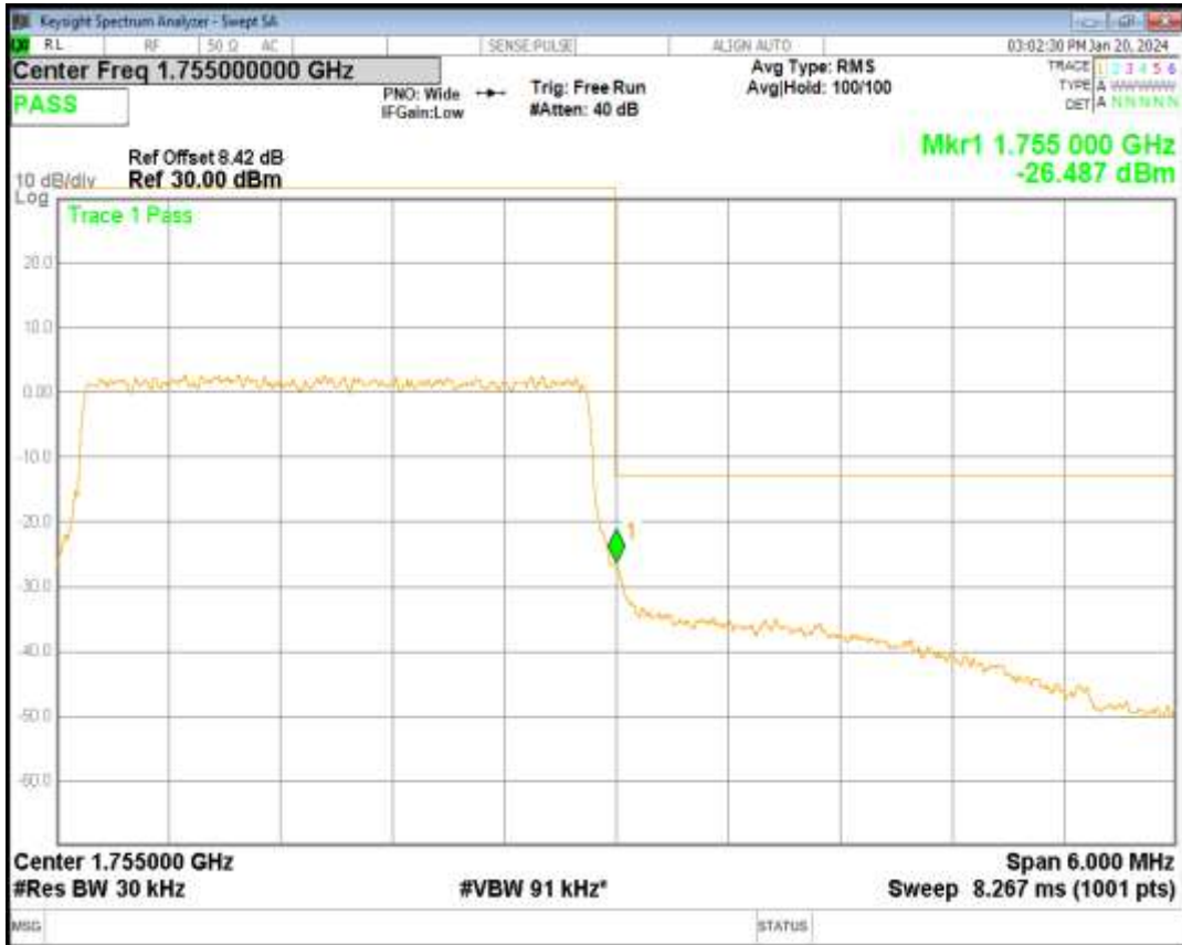
Band4 QPSK BW=10MHz Channel=20000 RB Size=50 Position=#0
