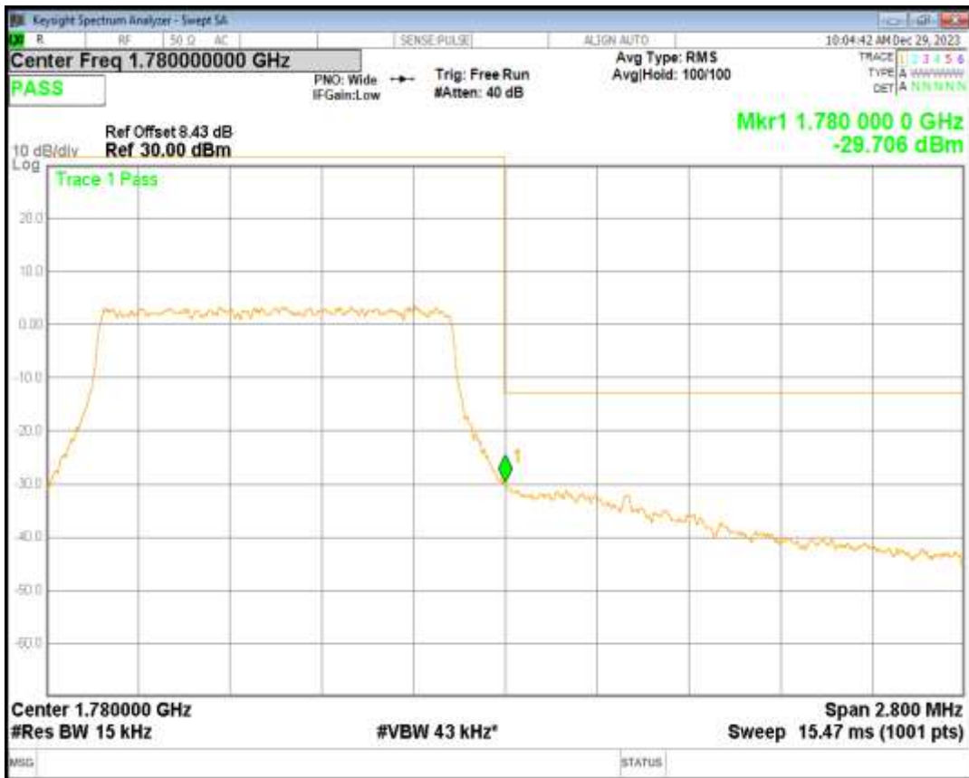
Band66 16QAM BW=10MHz Channel=132022 RB Size=50 Position=#0
