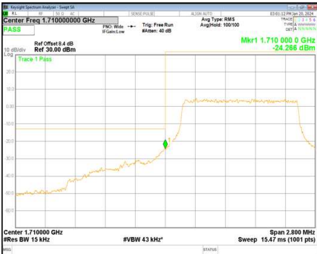
Band4 QPSK BW=10MHz Channel=20350 RB Size=50 Position=#0
