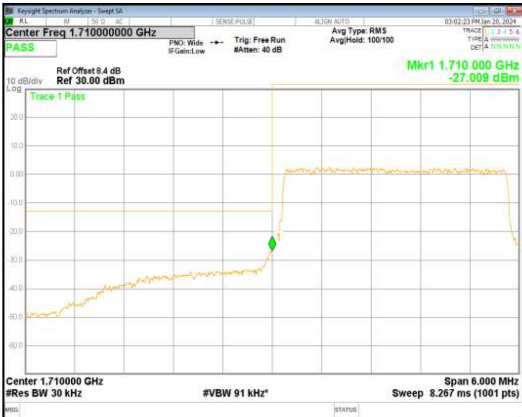
Band4 16QAM BW=3MHz Channel=20385 RB Size=15 Position=#0
