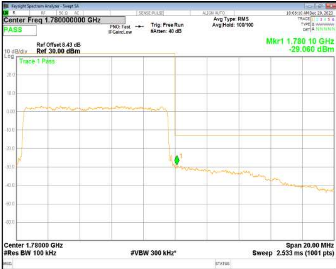
Band66 QPSK BW=15MHz Channel=132047 RB Size=75 Position=#0
