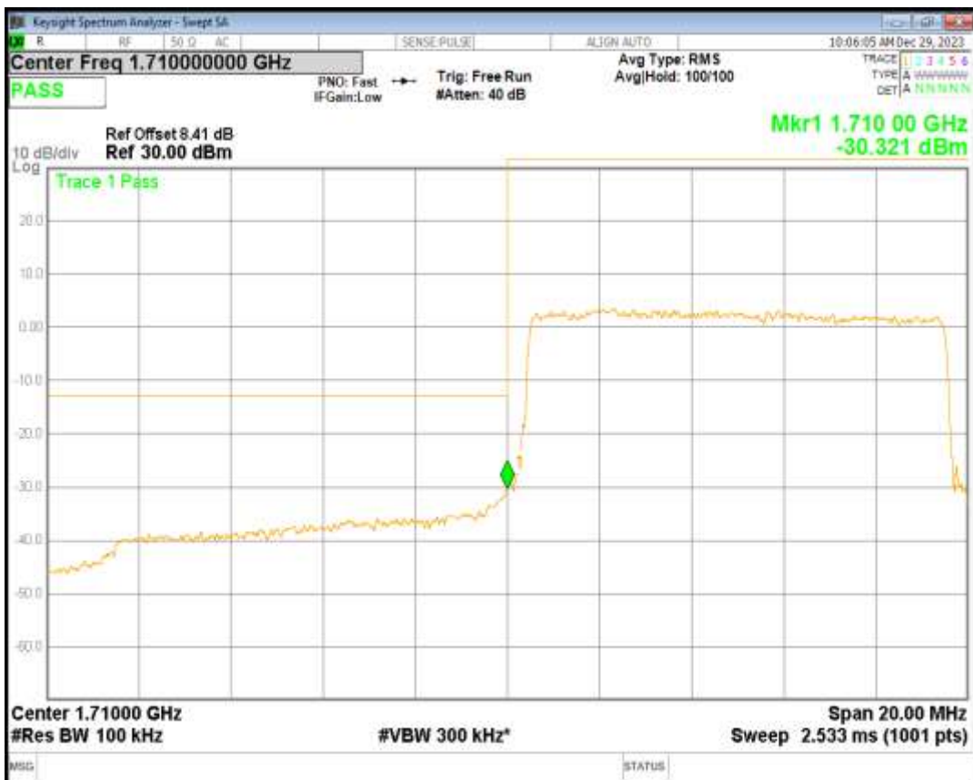
Band66 QPSK BW=10MHz Channel=132622 RB Size=50 Position=#0
