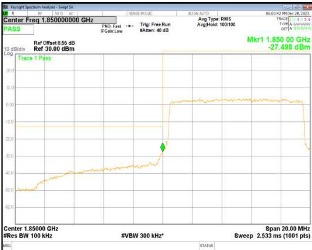
Band2 QPSK BW=10MHz Channel=19150 RB Size=50 Position=#0
