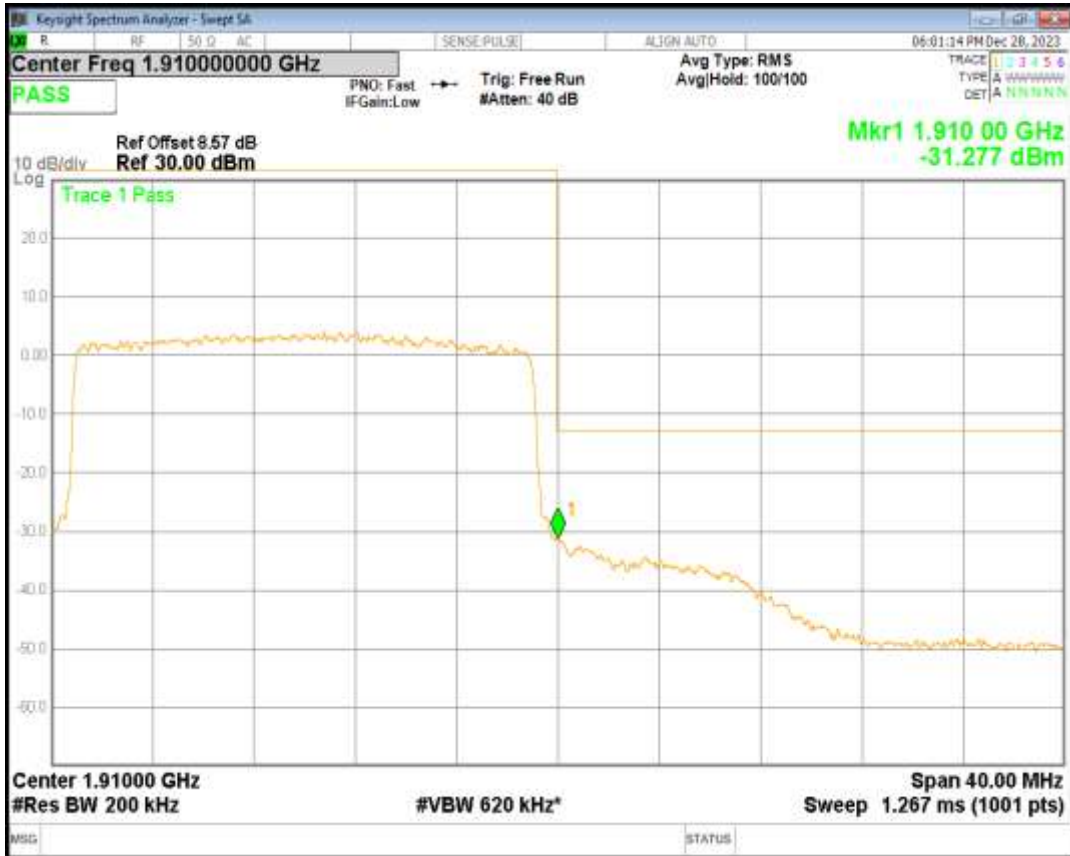
Band2 QPSK BW=3MHz Channel=18615 RB Size=15 Position=#0
