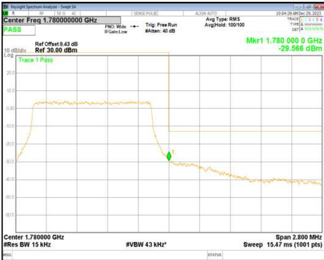
Band66 QPSK BW=10MHz Channel=132022 RB Size=50 Position=#0
