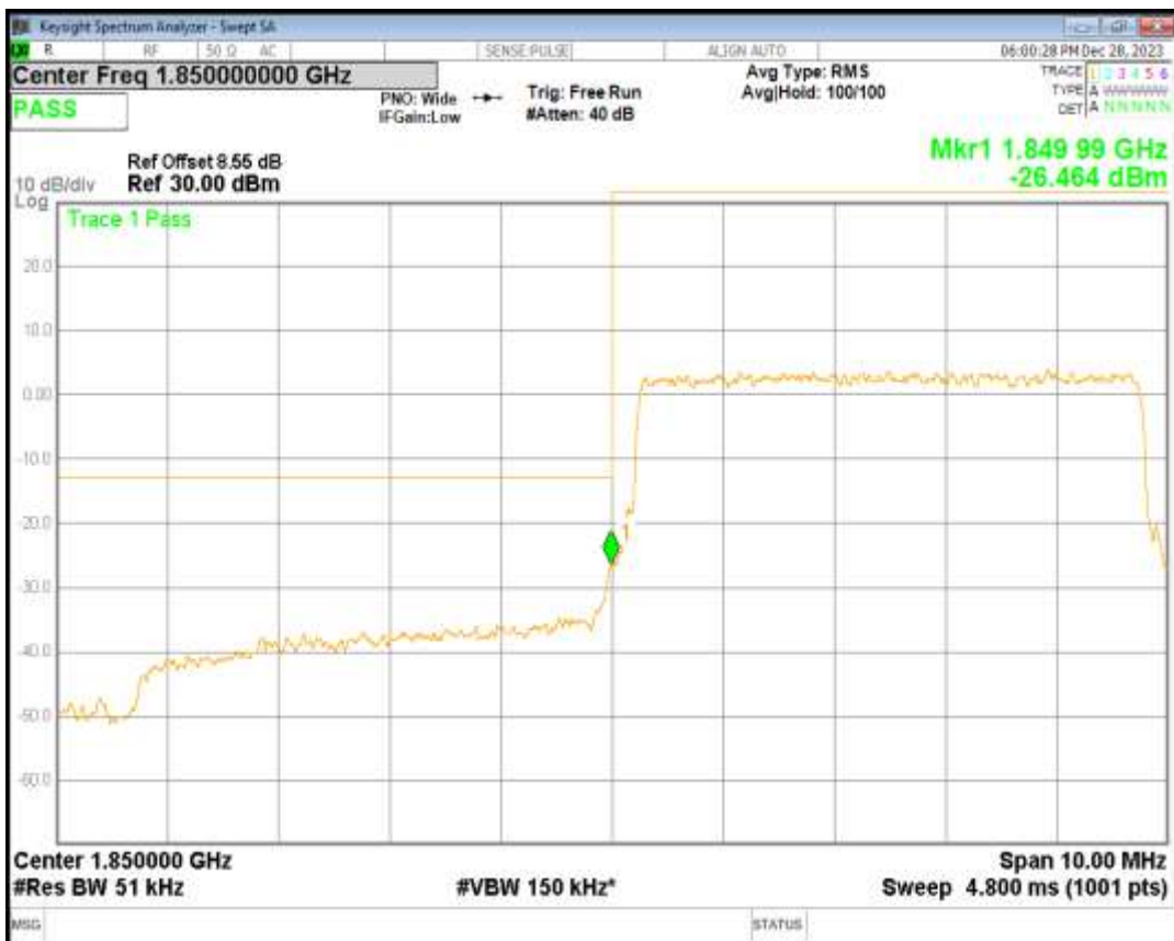
Band2 QPSK BW=5MHz Channel=19175 RB Size=25 Position=#0
