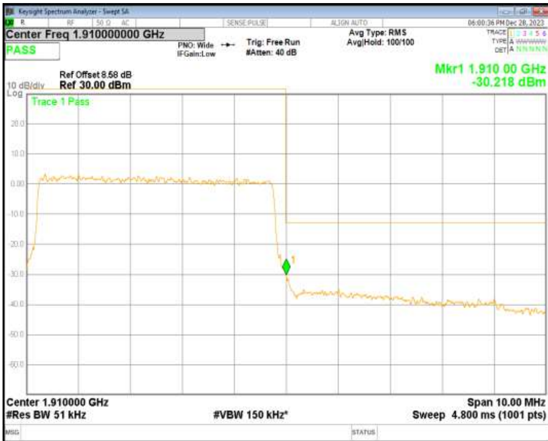
Band2 QPSK BW=1.4MHz Channel=18607 RB Size=6 Position=#0
