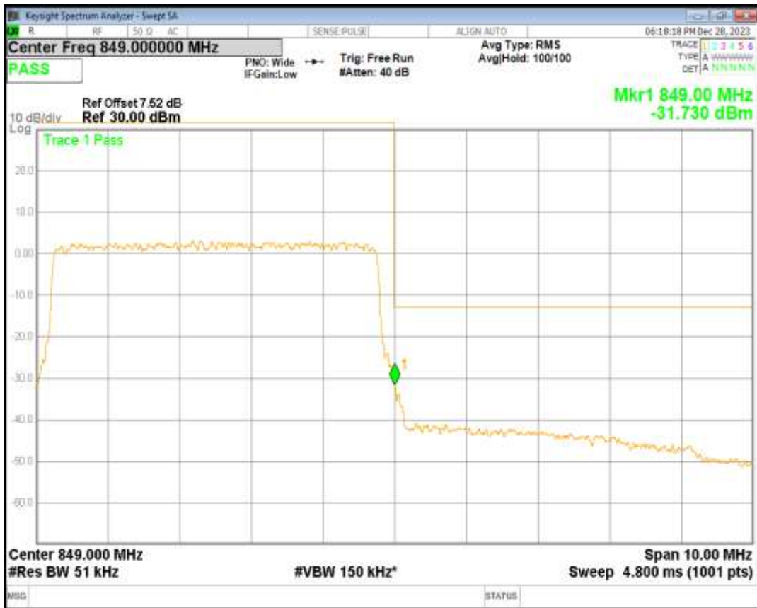
Band5 QPSK BW=1.4MHz Channel=20407 RB Size=6 Position=#0
