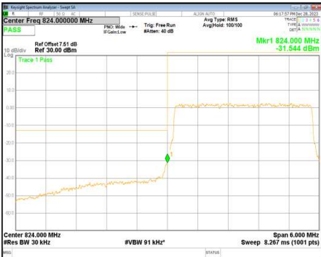
Band5 16QAM BW=3MHz Channel=20635 RB Size=15 Position=#0
