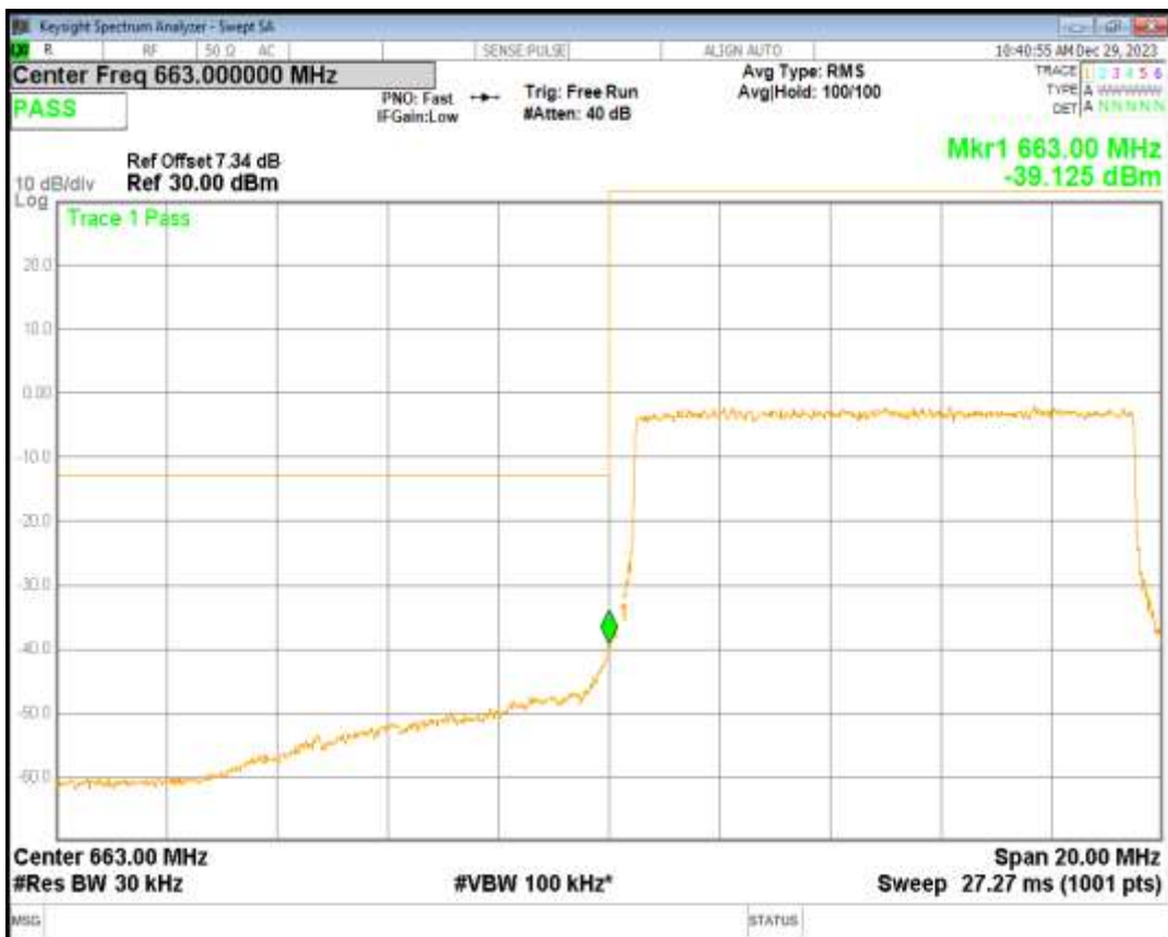
Band71 16QAM BW=10MHz Channel=133422 RB Size=50 Position=#0
