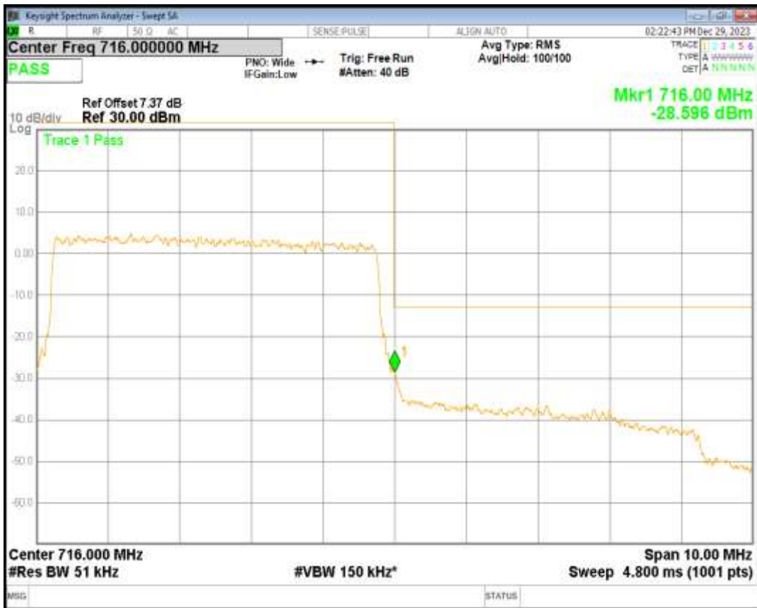
Band2 16QAM BW=1.4MHz Channel=18607 RB Size=6 Position=#0
