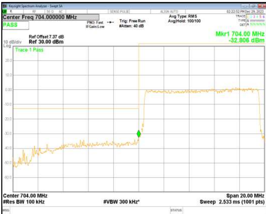
Band17 QPSK BW=10MHz Channel=23800 RB Size=50 Position=#0
