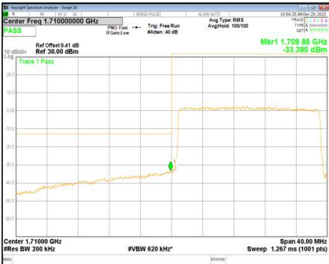
Band66 16QAM BW=20MHz Channel=132572 RB Size=100 Position=#0
