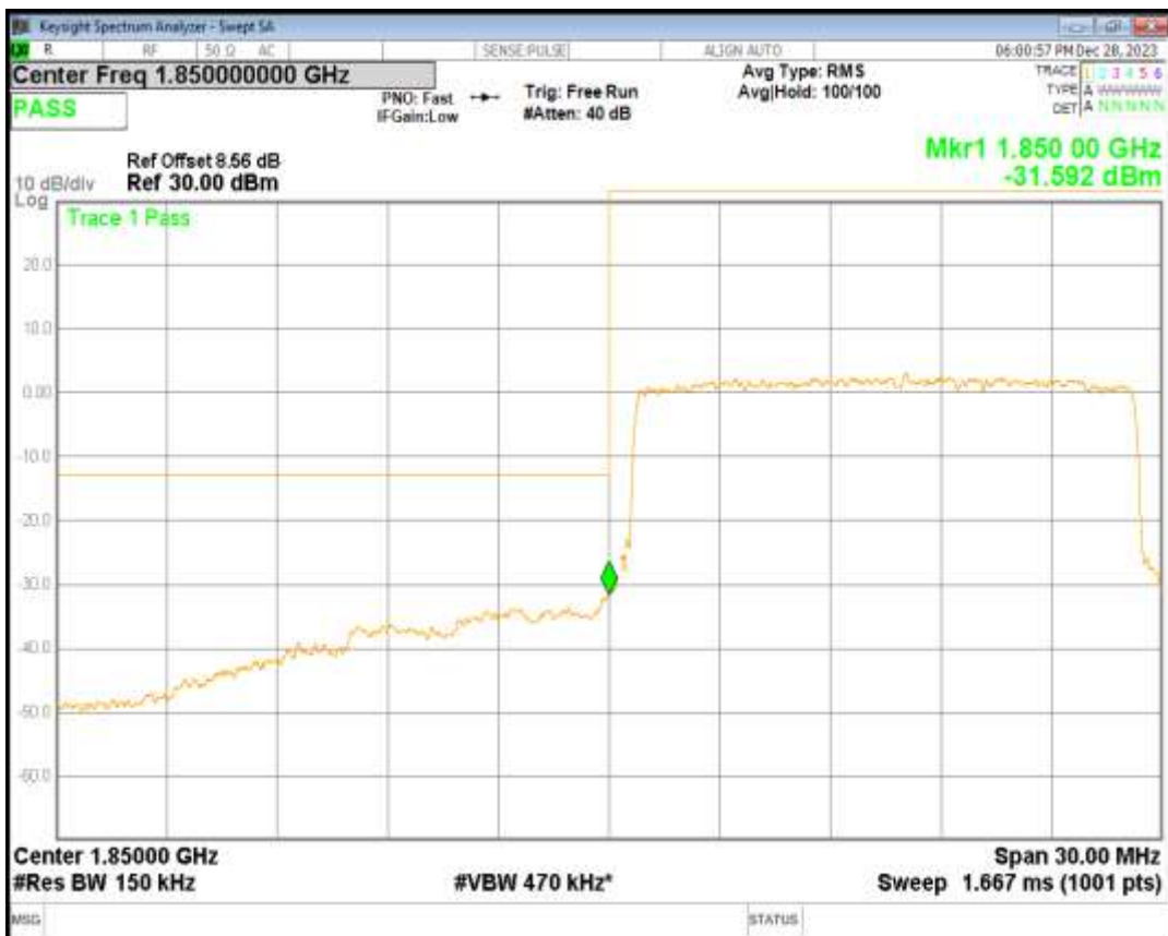
Band2 16QAM BW=15MHz Channel=19125 RB Size=75 Position=#0
