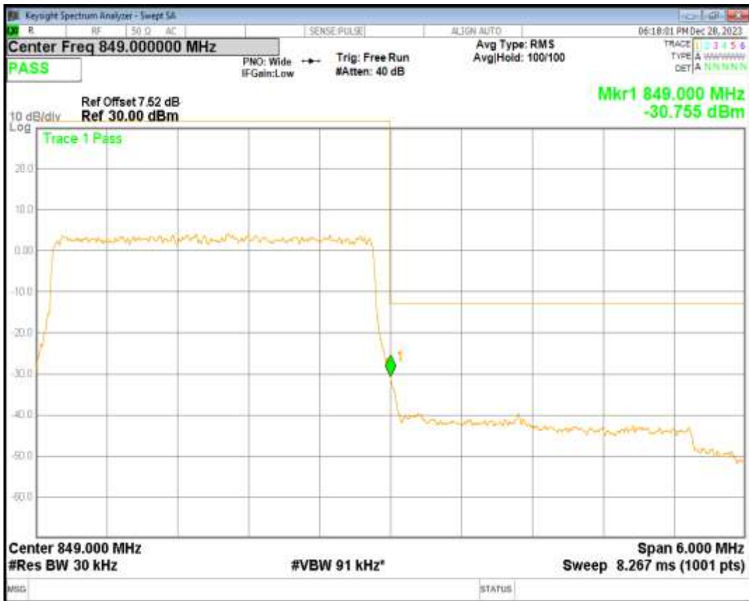
Band5 QPSK BW=5MHz Channel=20425 RB Size=25 Position=#0
