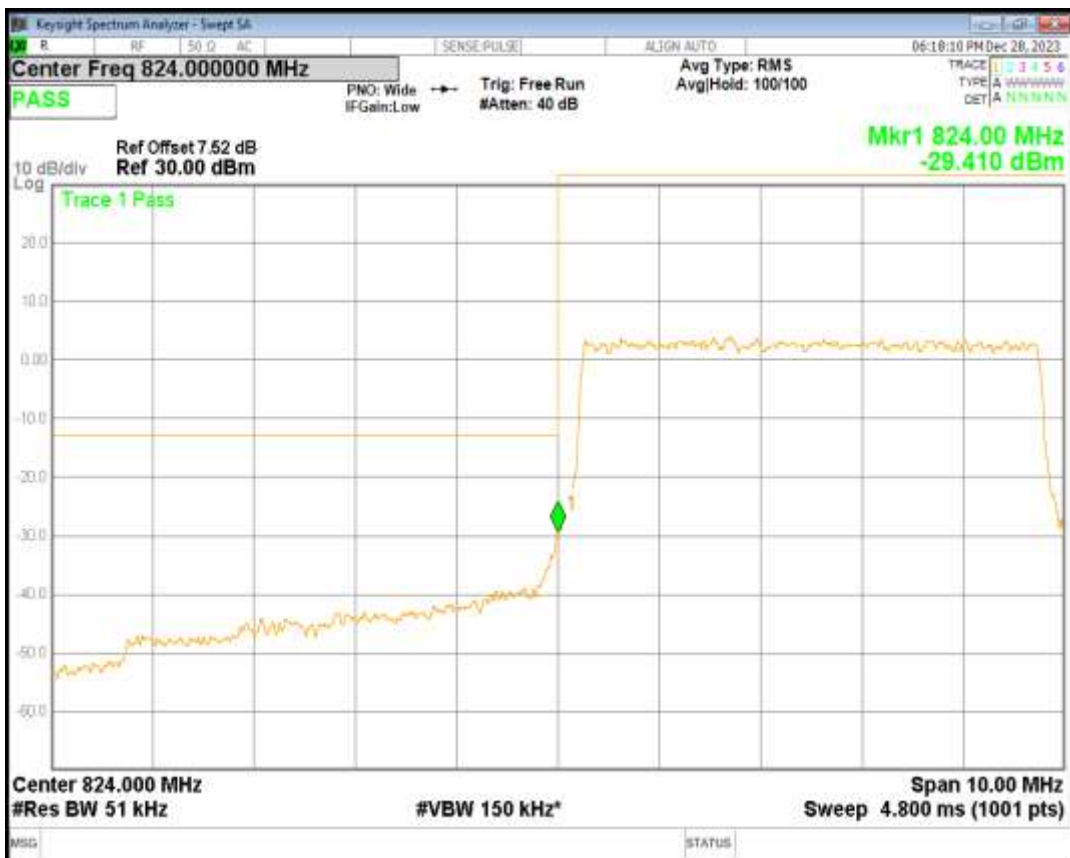
Band5 QPSK BW=5MHz Channel=20625 RB Size=25 Position=#0
