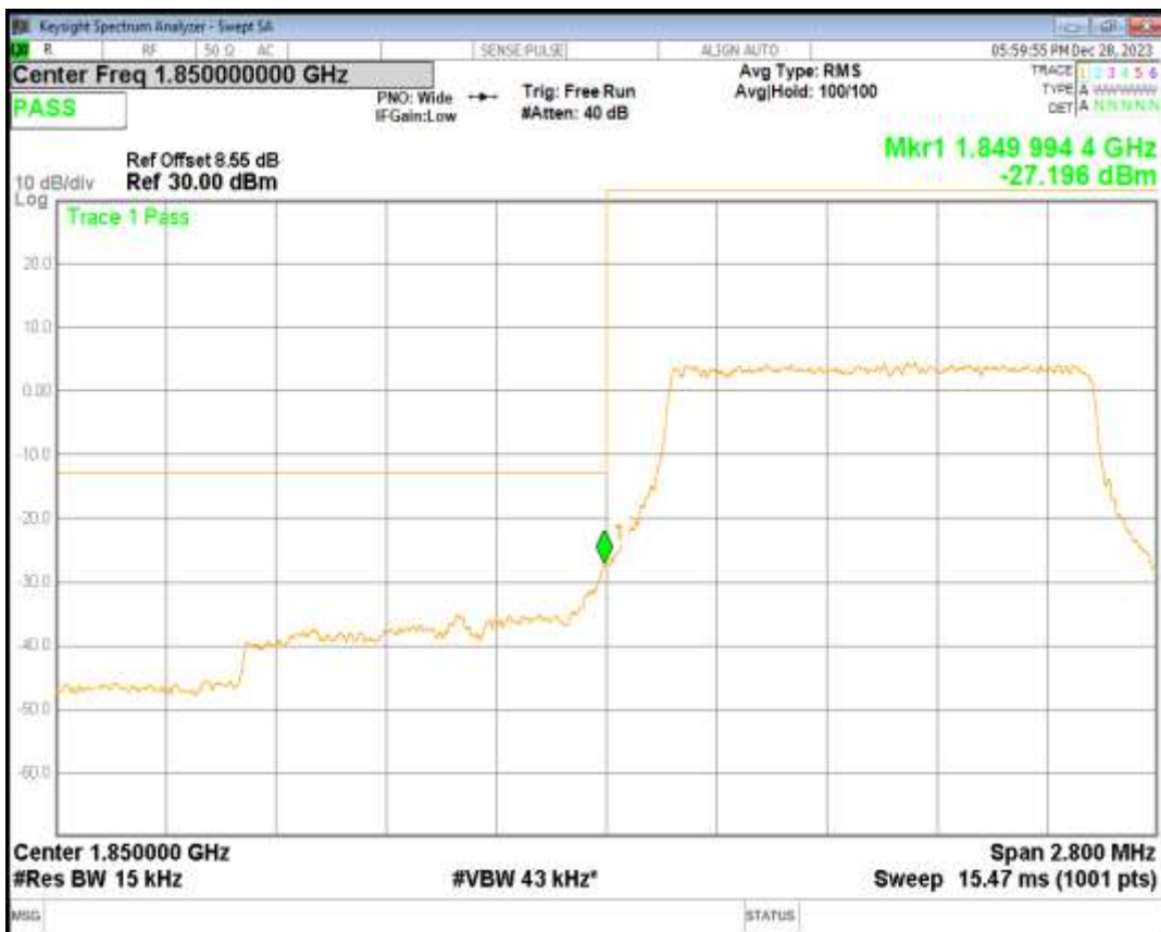
Band2 QPSK BW=1.4MHz Channel=19193 RB Size=6 Position=#0
