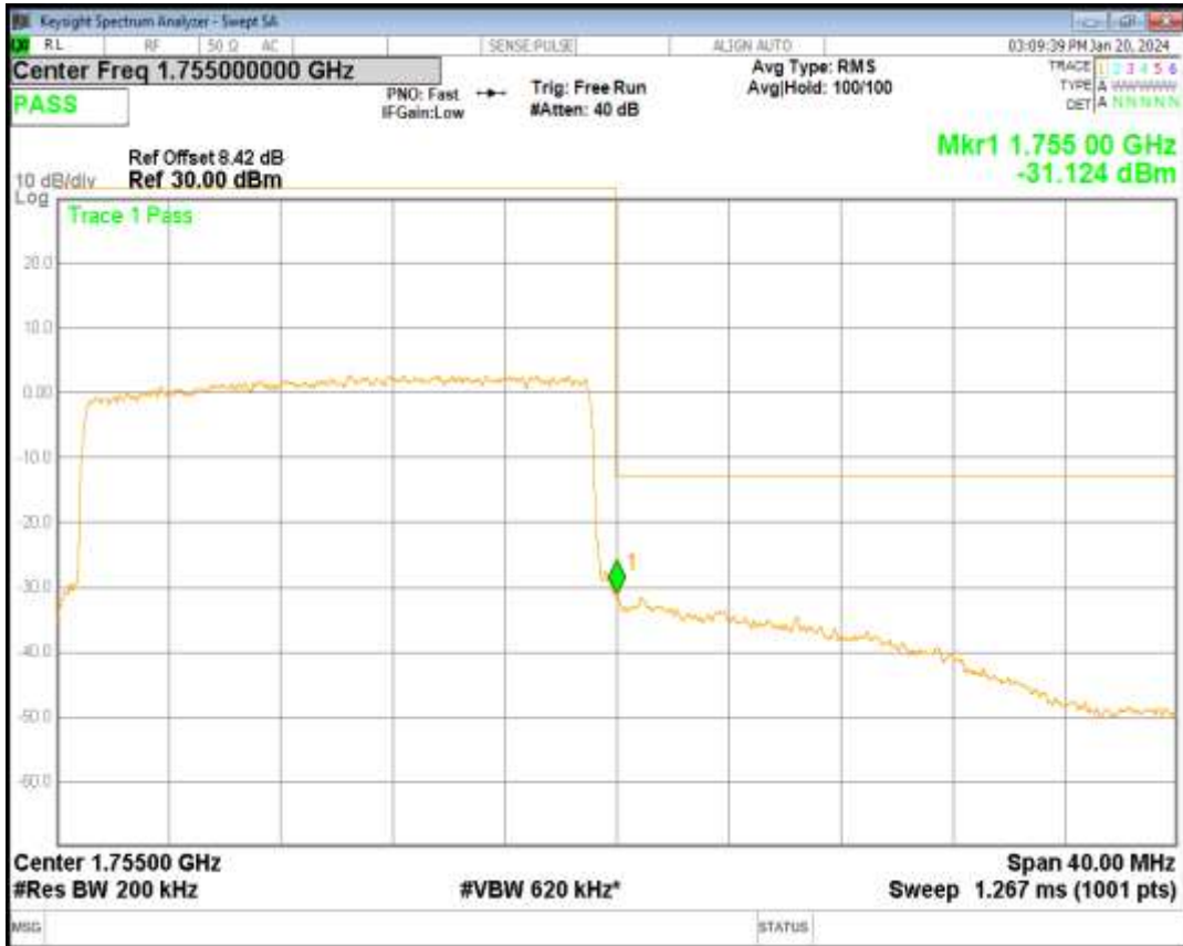
Band4 16QAM BW=3MHz Channel=19965 RB Size=15 Position=#0
