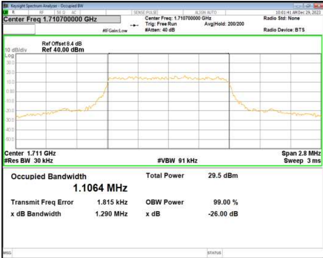
Band66 QPSK BW=1.4MHz Channel=132322 RB Size=6 Position=#0
