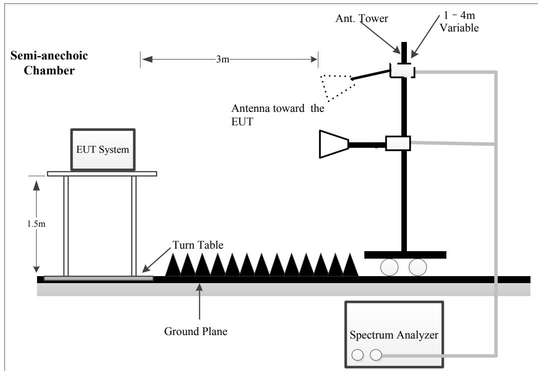
The radiated emissions were performed in the 3 meters distance, using the setup accordance with the ANSI C63.10-2013. The specification used was the FCC 15.209, and FCC 15.247 limits.
