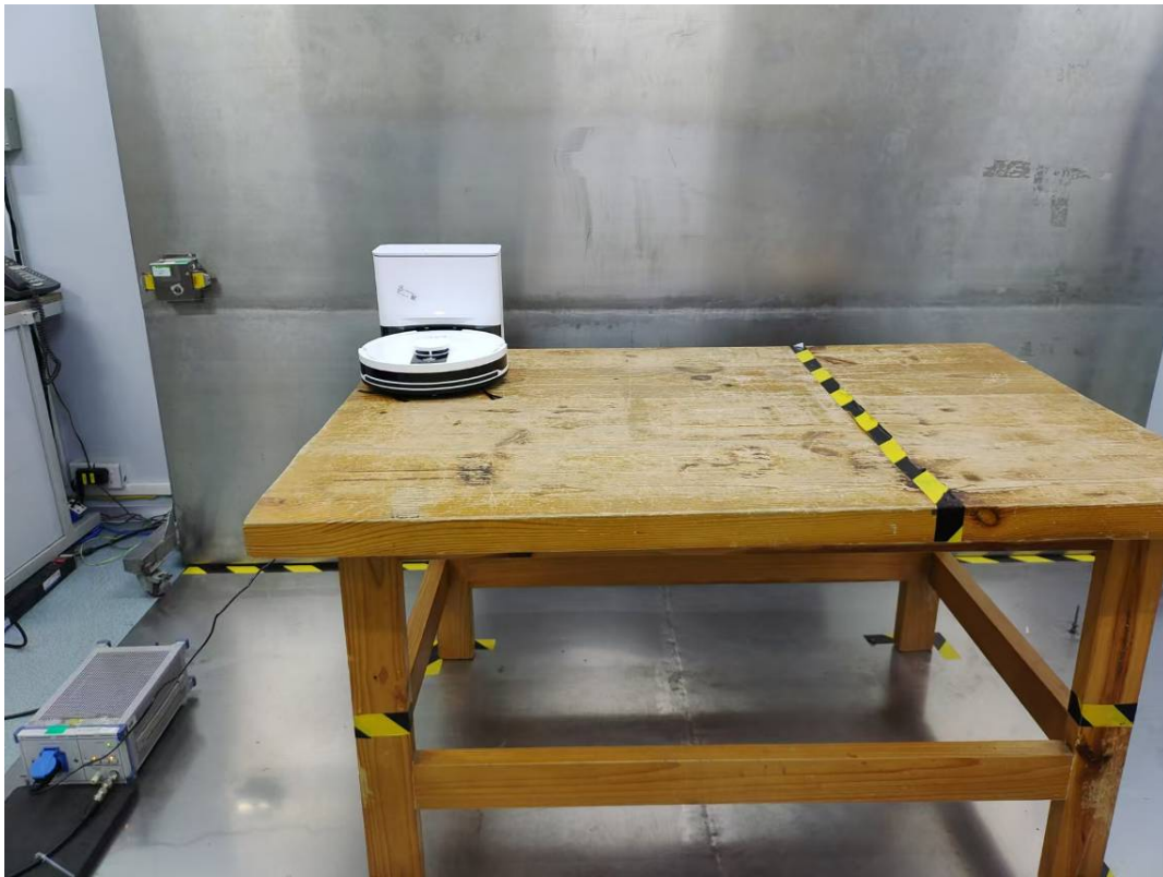
Conducted Emissions Side View-M1&M2
