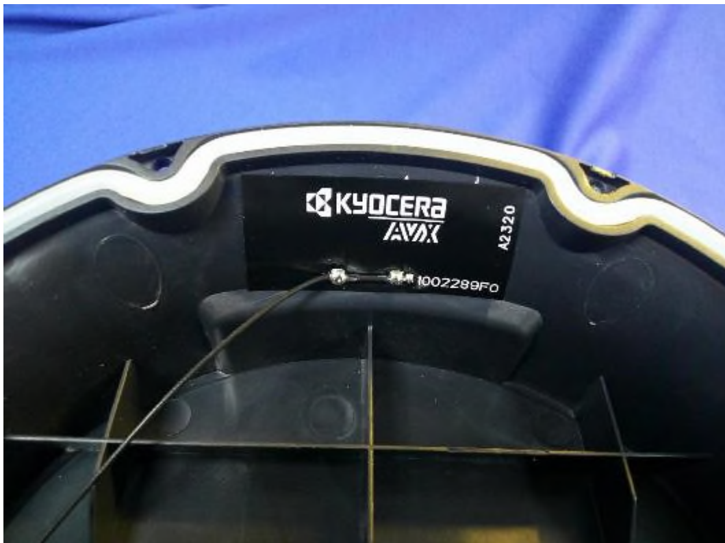
Photograph shows the EUTs cellular antenna
