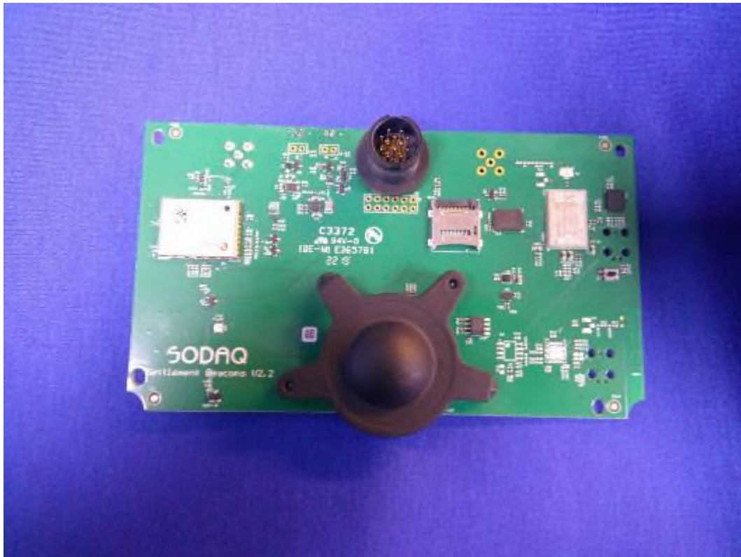
Photograph shows the EUTs 60GHz RADAR antenna with lens fitted
