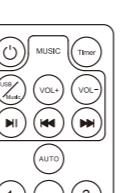
① Power on/off ② Play/pause ③ Previous song ④ Next song ⑤ Volume up ⑥ Volume down ⑦ AUTO mode: press to enter AUTO mode/gear 2 with timer 15 minutes ⑧ Stop swing: press to stop swing, and press any gear key to resume swing.
