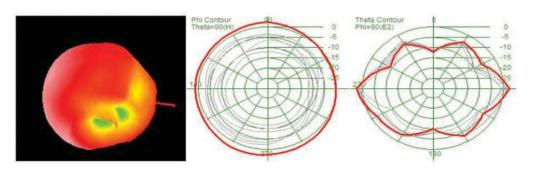
433.92MHz Peak Gain: 0 dBi Efficiency:50.1%
