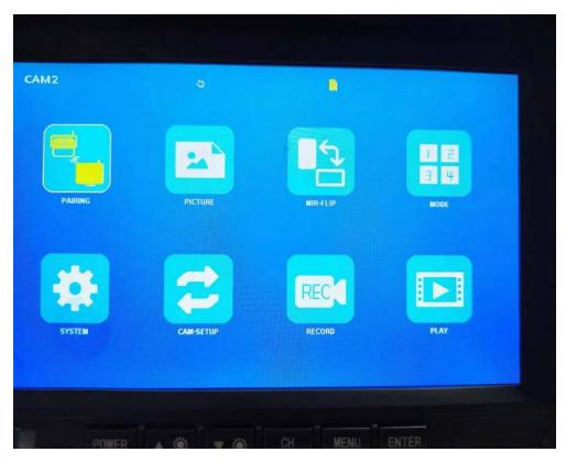
Enter the code mode, 20 seconds of code countdown. At the same time, the launch side is in the code strong state to pair the code.
