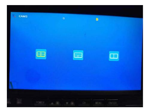
5. Camera setting: Under this menu, you can choose the switch status of the four cameras, the cycle time, and set the automatic cycle.
