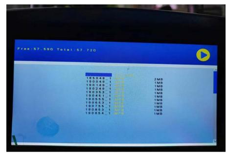
8. Video Settings: enter the video Settings interface, you can format the SD card and loop video function. Note: The first use of a new card must be formatted in this machine for normal use.
