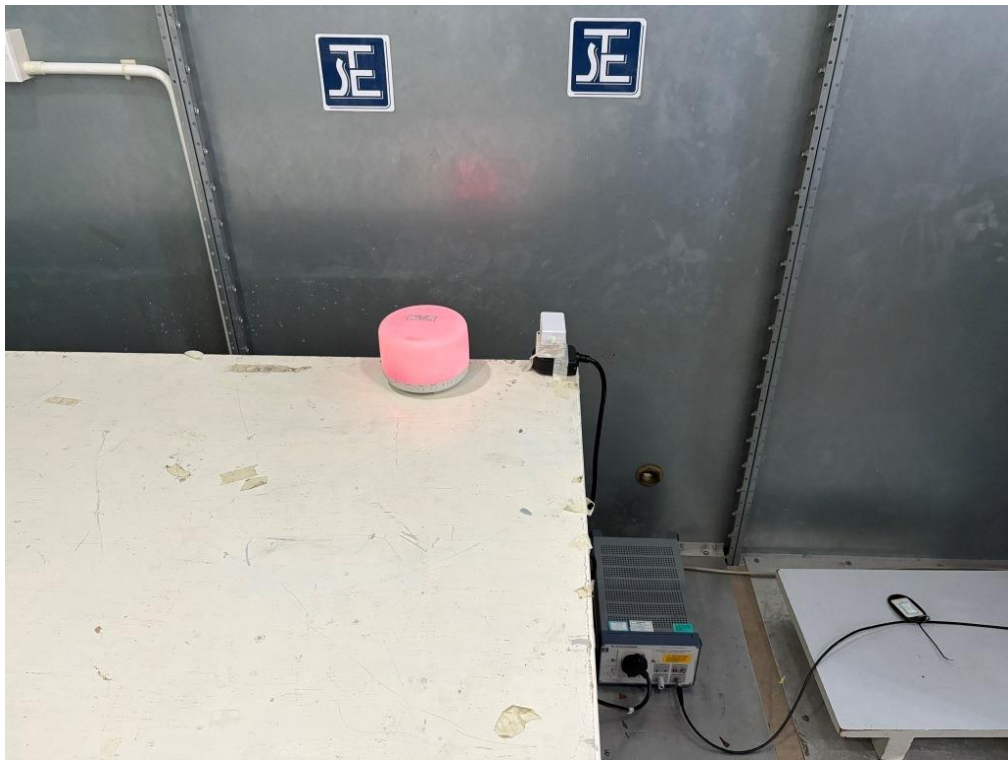
Measurement of Conducted Emission Test Set Up
