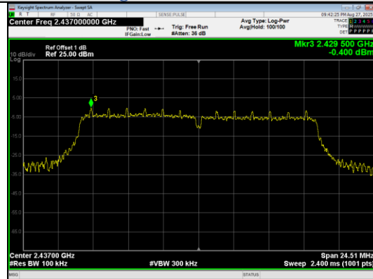
In-Band Reference Level IEEE 802.11g Channel 6_20MHz_Antenna 0
