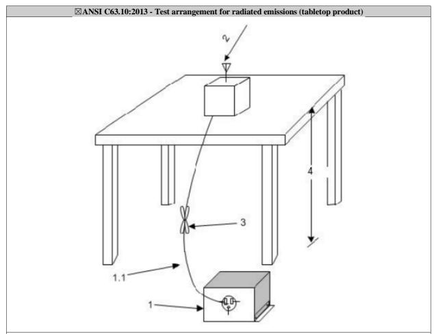
1—A LISN is optional for radiated measurements between 30 MHz and 1000 MHz but not allowed for measurements below 30 MHz and above 1000 MHz. If used, then connect EUT to one LISN. Unused LISN measuring port connectors shall be terminated in 50  $\Omega$  loads. The LISN may be placed on top of, or immediately beneath, the reference ground plane.
