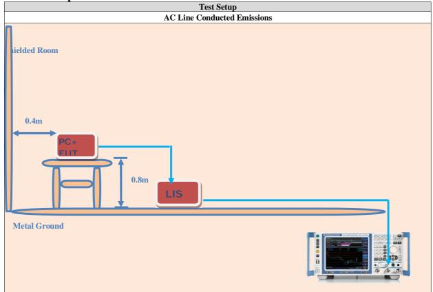
This test is applicable for radio equipment and/or ancillary equipment for fixed use powered by the AC mains. This test shall be performed on a representative configuration of the radio equipment, the associated ancillary equipment, or a representative configuration of the combination of radio and ancillary equipment. This test assesses the level of internally generated electrical noise present on the AC power input/output ports.
