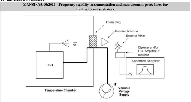
The following procedure shall be used for determining frequency stability of millimeter-wave systems:
