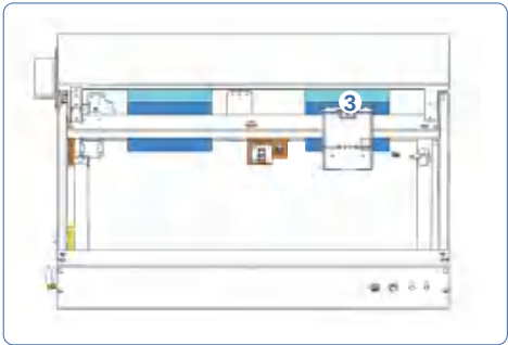
Move the X-axis forward and then take out the foam 3
