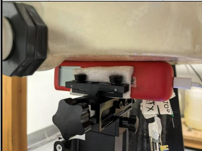
Right Side of EUT with 0mm Gap
