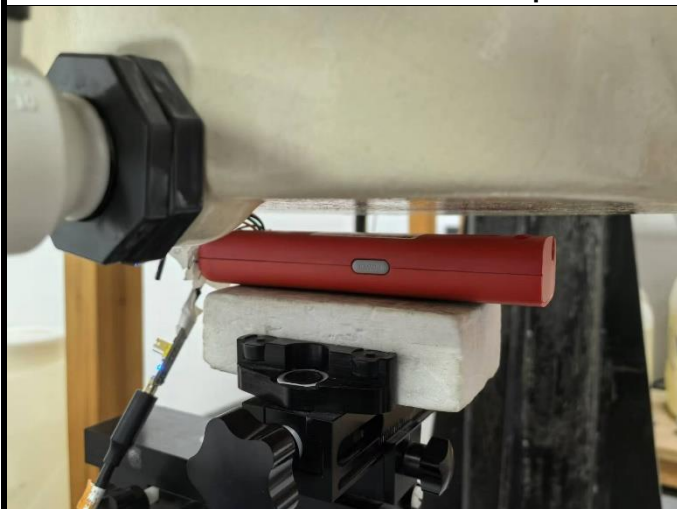
Rear Face of EUT with 10 mm Gap
