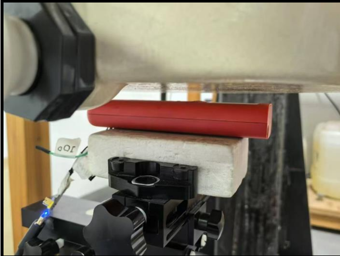
Front Face of EUT with 10 mm Gap
