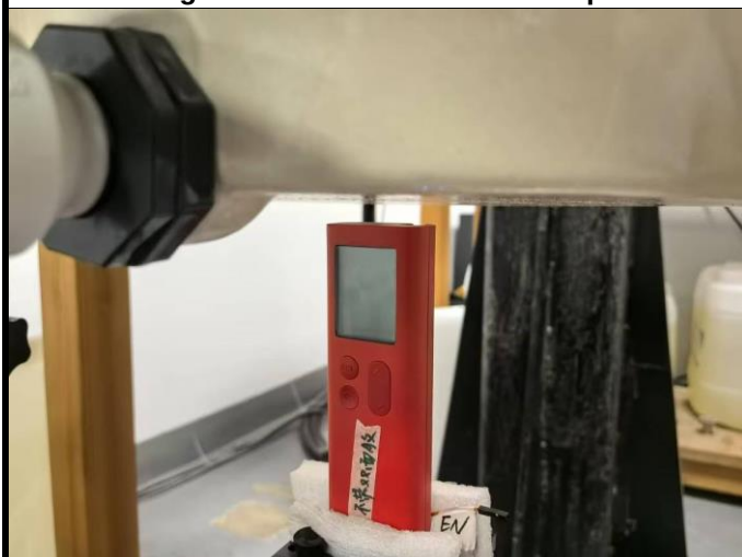
Top Side of EUT with 10mm Gap
