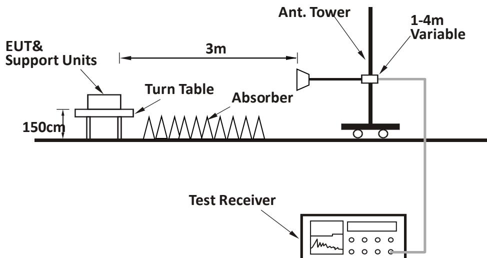
**TEST REPORT****3.4 Test Results of Radiated Emissions**
