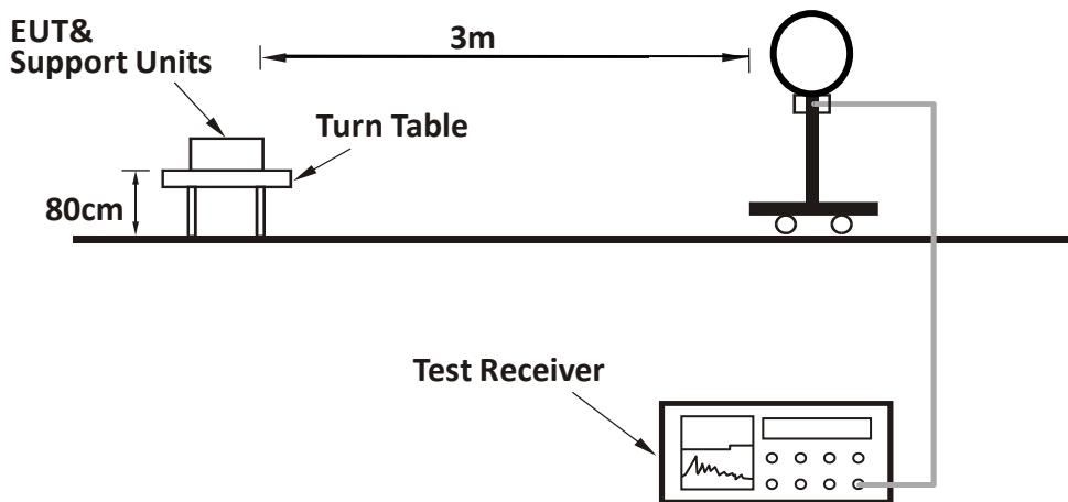
**For Radiated emission 30MHz to 1GHz:**
