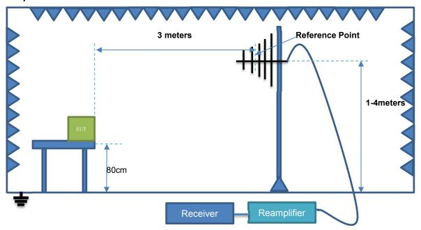
Radiation Test (30MHz - 1GHz)
