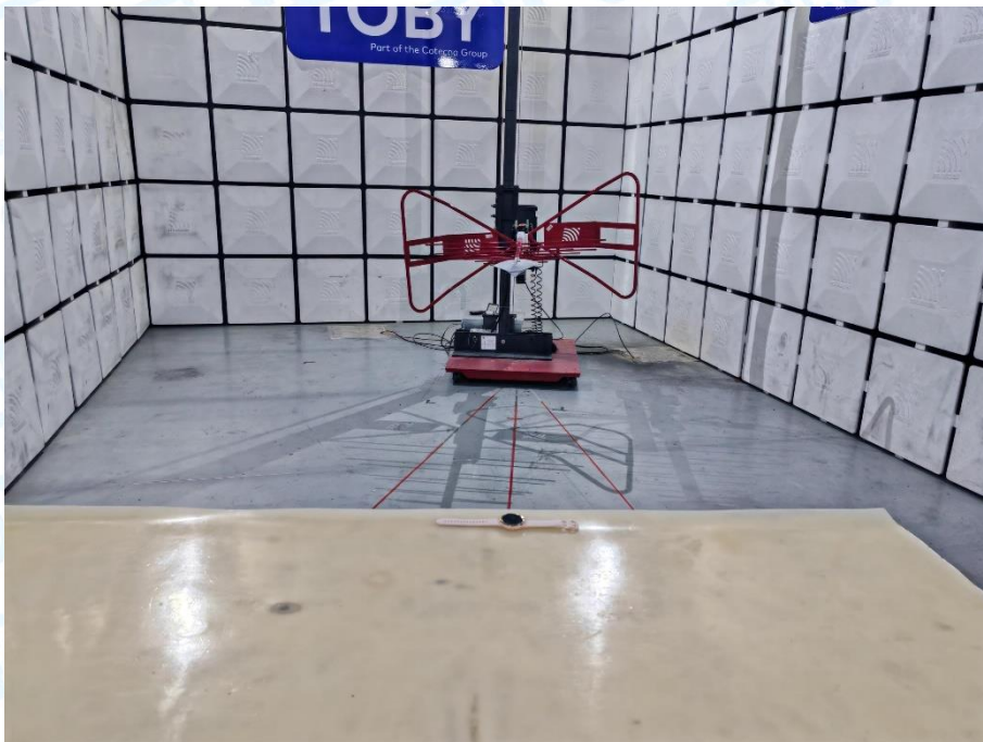
Photo of Setup for Radiated Emission (30MHz~1GHz)
