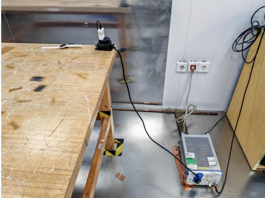
Photo of Setup for Radiated Emission (30MHz~1GHz)
