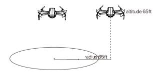
Second-level low battery: The aircraft will directly descend from its current altitude to the ground.
