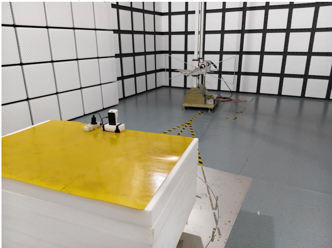
Radiated Spurious Emissions Test View (30MHz-1GHz) (Test Mode 1)
