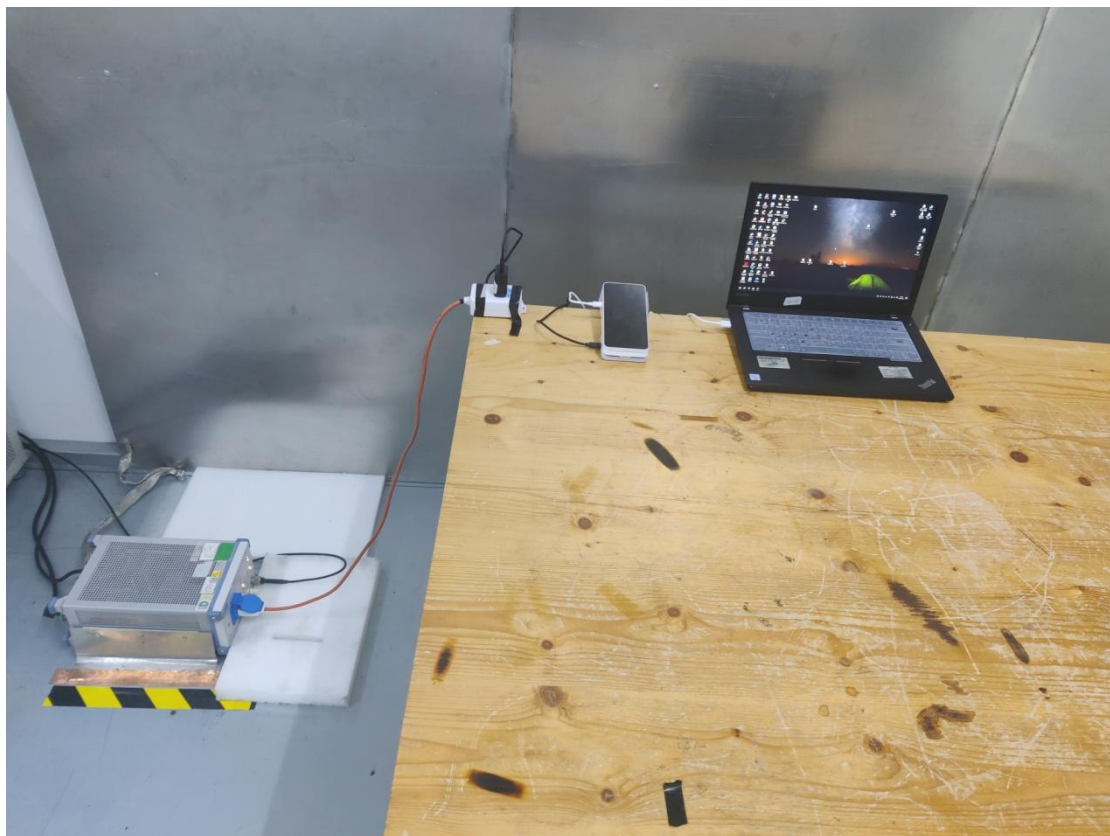
Photo of Power Line Conducted Emission Measurement-Front View(Test Mode 4)
