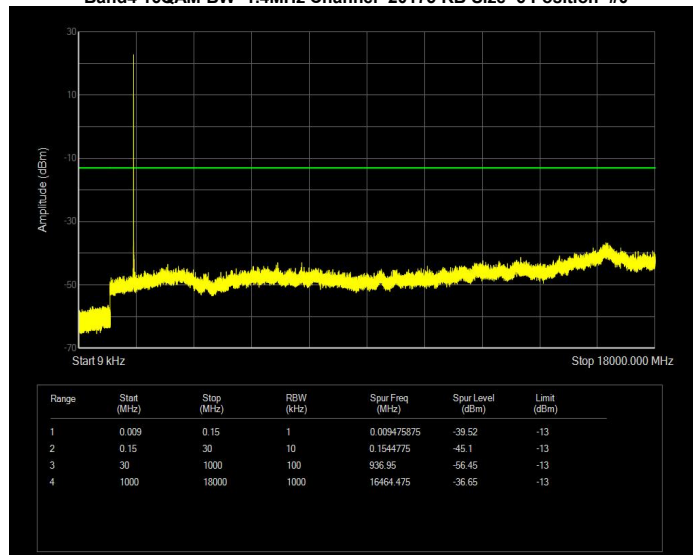
Band4 16QAM BW=1.4MHz Channel=20393 RB Size=6 Position=#0
