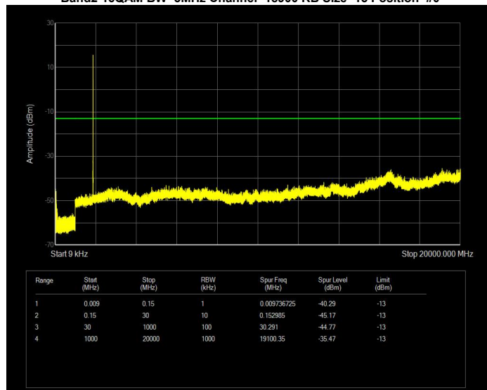
Band2 16QAM BW=3MHz Channel=19185 RB Size=15 Position=#0
