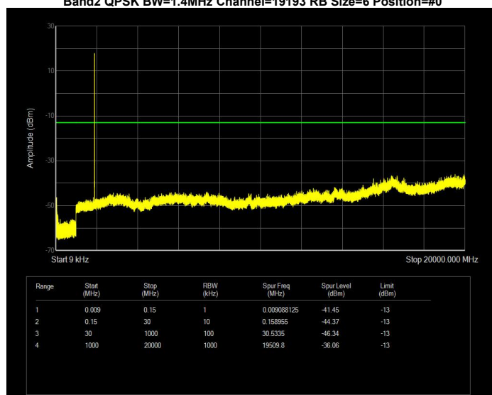
Band2 QPSK BW=1.4MHz Channel=19193 RB Size=6 Position=#0
