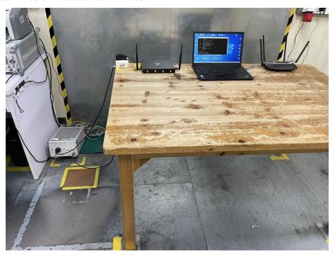
Spurious Emission Test Setup (Below 1GHz)
