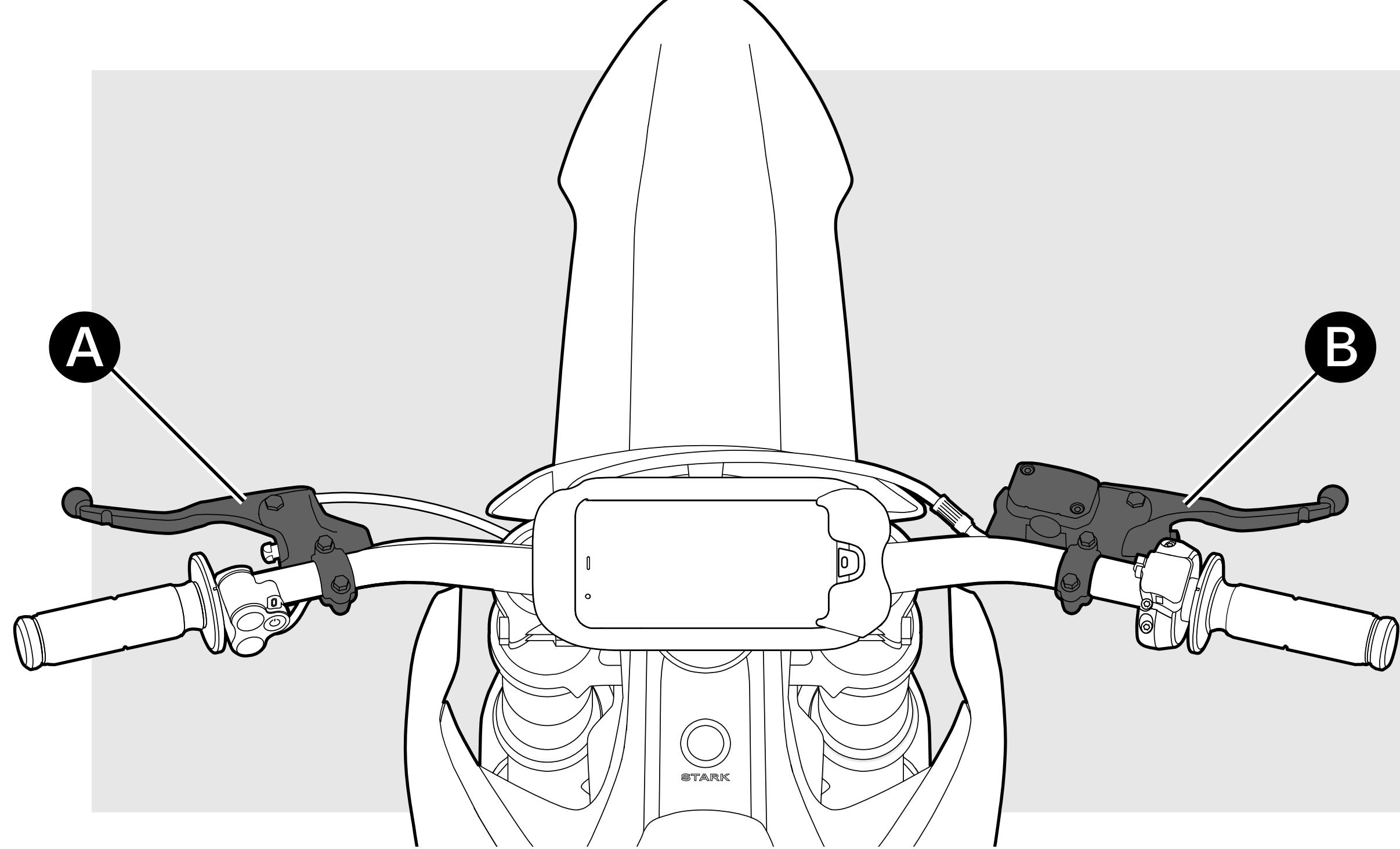
A Rear hand brake      B Front brake
