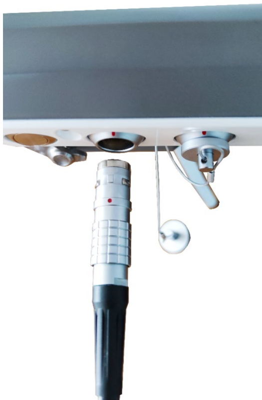
Figure 5-4 Connect the power Cable (Aim at the red dot)
