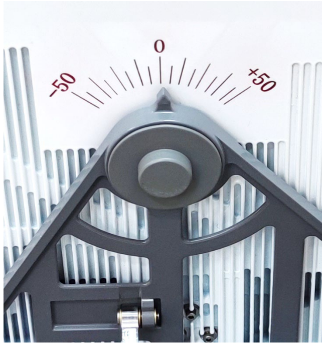
Figure 8-3 Polarization Adjustment Scale and Indicator
